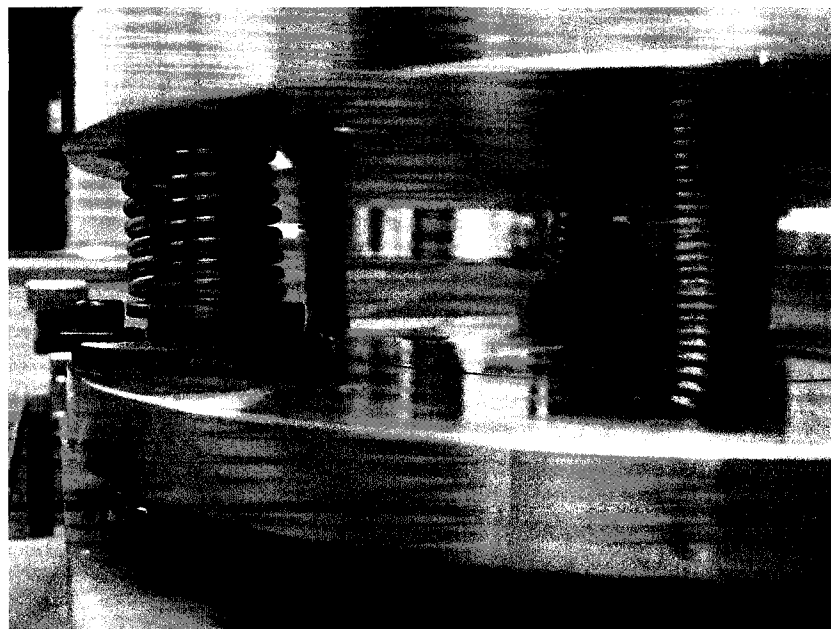
Figure 4.30: Compression springs in the fully compressed state, such that the applied force is maximum
