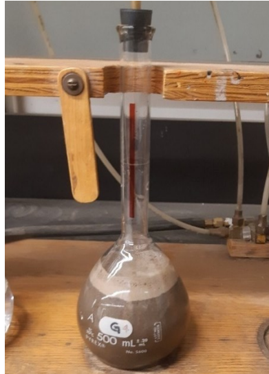
Figure 4.4. Vacuum procedure in soil mixture for specific gravity test.
