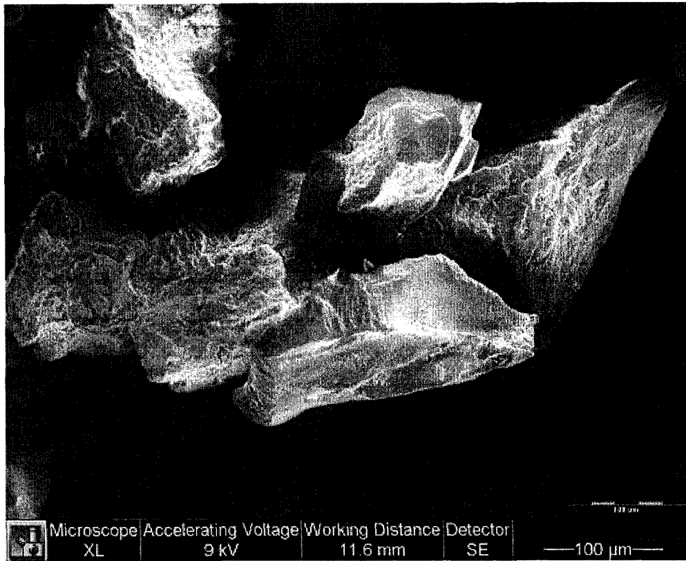
Figure 7.3 SEM of reconstituted (washed) oil sand sample at high resolution (573×431 μm 2 viewing area)
