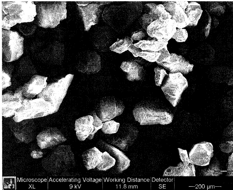
Figure 7.2 SEM of reconstituted (washed) oil sand sample ( 1433 \times 1075 \mu\text{m}^2 viewing area)
