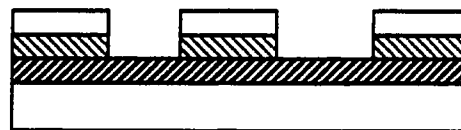
( c ) The exposed Au is removed using commercial aqua regia
