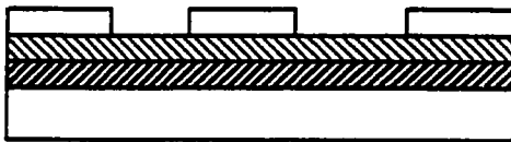
( b ) The photoresistant is exposed to UV light thereby removing the desired region
