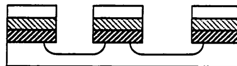
( e ) The exposed glass is etched using \text{HF}/\text{HNO}_3/\text{H}_2\text{O}
