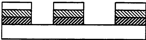
( d ) The exposed Cr is removed using commercial Cr etch
