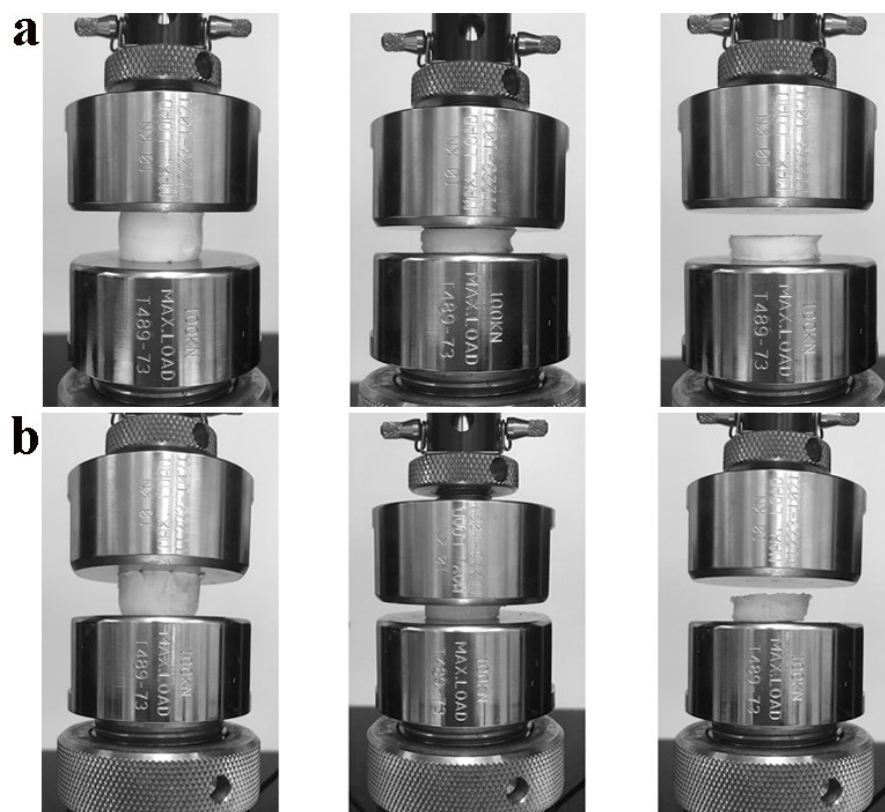
Figure S 4 Compression images of the Aerogel-6 (a) and PVA-ECH sponge (b).
