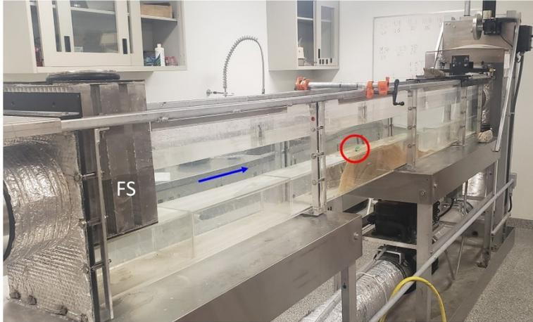
Figure 2.4 A photograph of the recirculating flume set up for the transport and feeding experiments. The flow straightener (FS) is situated on the left. The blue arrow indicates flow direction when in operation. A green PLA brachiopod model in the sand is circled in red. The impeller which generates flow is situated on the right. Return flow passes underneath the working chamber.
