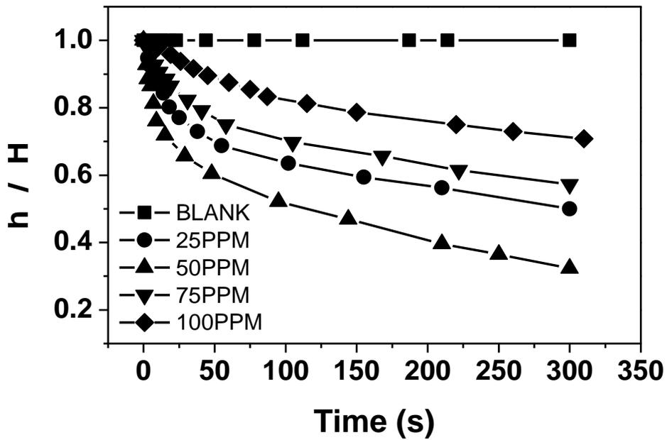
**Figure 3.8** Settling curves of diluted MFT (5 wt% solids) with Al-PAM as flocculant
