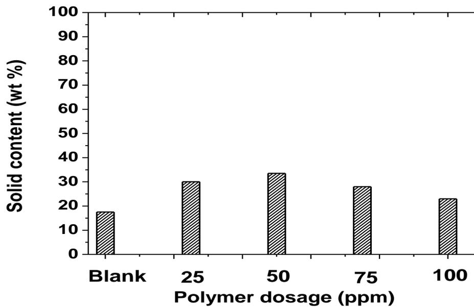
**Figure 3.22** Solid content of the sediment formed by settling of MFT diluted 5 wt% solids with MF1011 as flocculant
