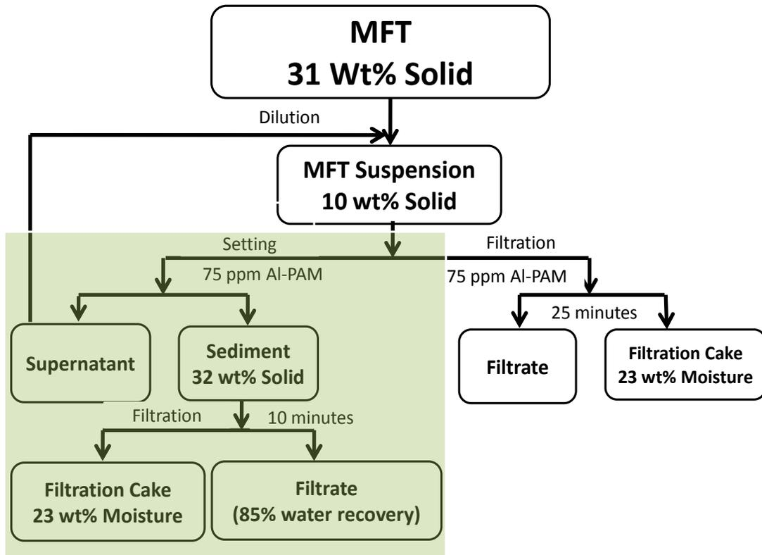
**Figure 4.1** Schematic flow diagram of a single stage filtration (plain section) and two stage (shaded section) filtration of flocculated sediment
