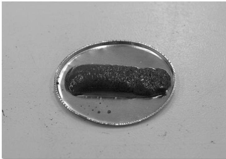
**Figure 3.25** Sediments obtained under optimum conditions for Al-PAM (32 wt% solids)
