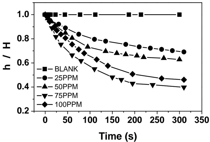
**Figure 3.6** Settling curves of diluted MFT (10 wt% solids) with Al-PAM as flocculant
