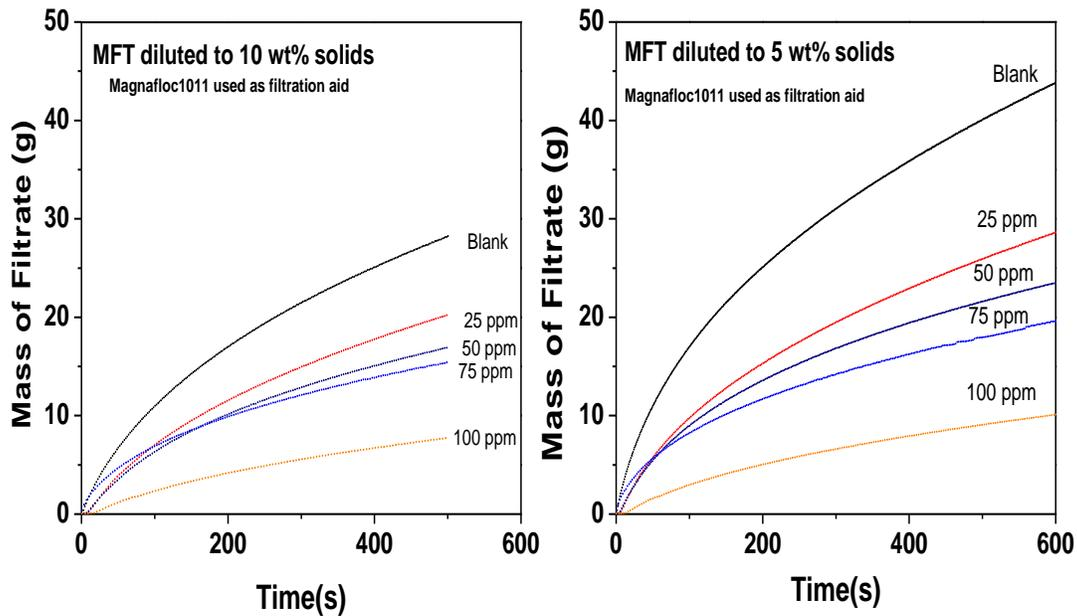
**Figure 3.26** Filtration rate of MFT diluted to 10 wt% and 5 wt% solids with MF1011 as filtration aid
