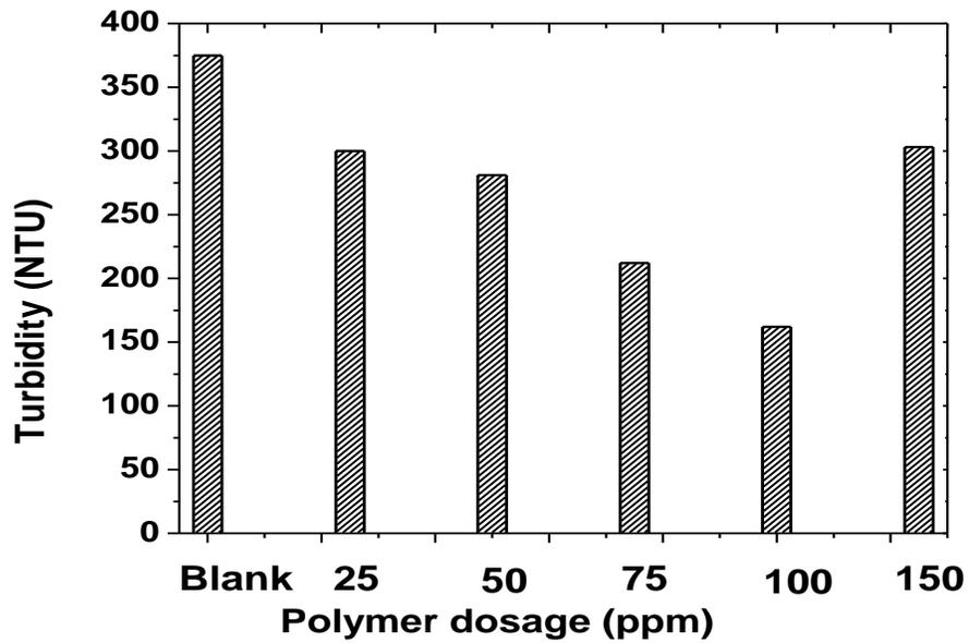
**Figure 3.11** Turbidity of supernatant recovered from MFT diluted to 10 wt% solids with MF1011 as flocculant
