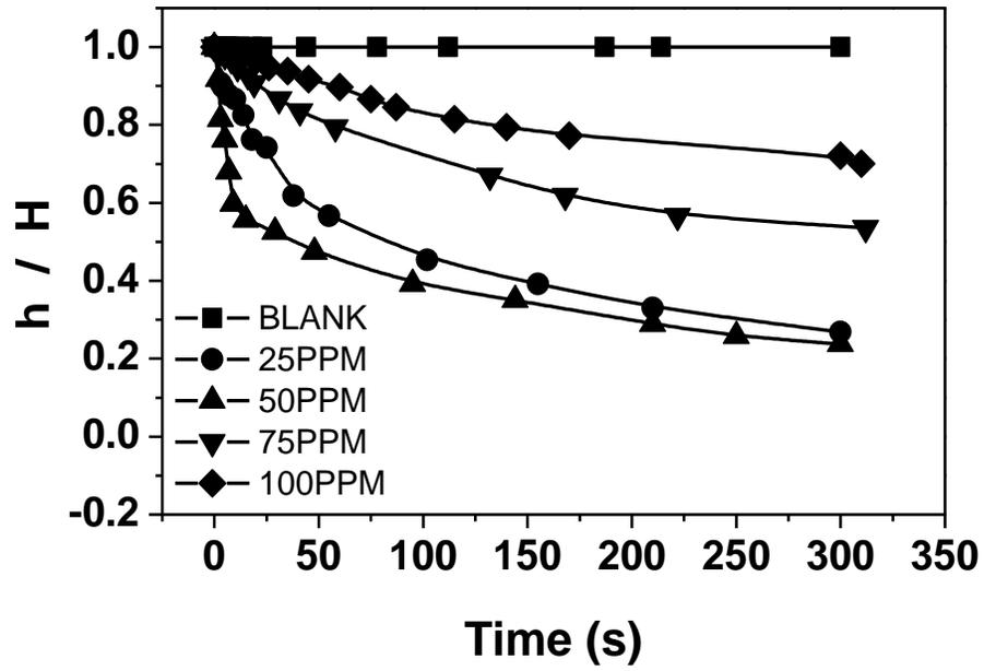
**Figure 3.7** Settling curves of diluted MFT (5 wt% solids) with MF1011 as flocculant
