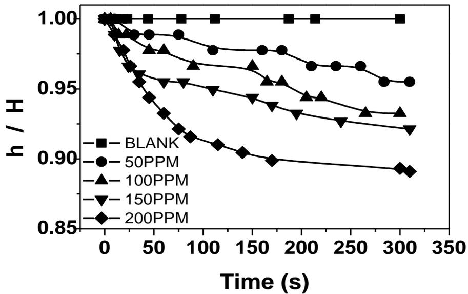
**Figure 3.2** Settling curves of raw MFT (31 wt% solids) with Al-PAM as flocculant
