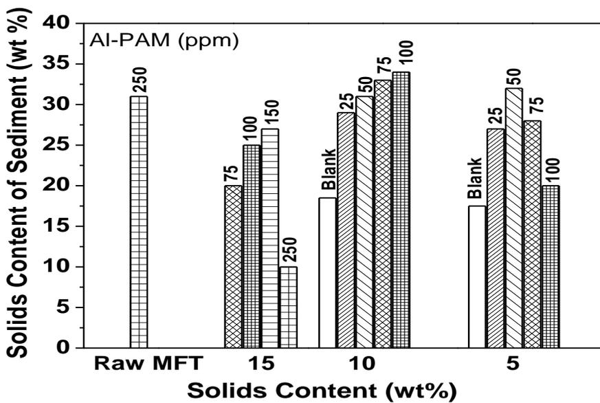
**Figure 3.20** Solid content of sediment after settling of undiluted and diluted MFT with Al-PAM as flocculant
