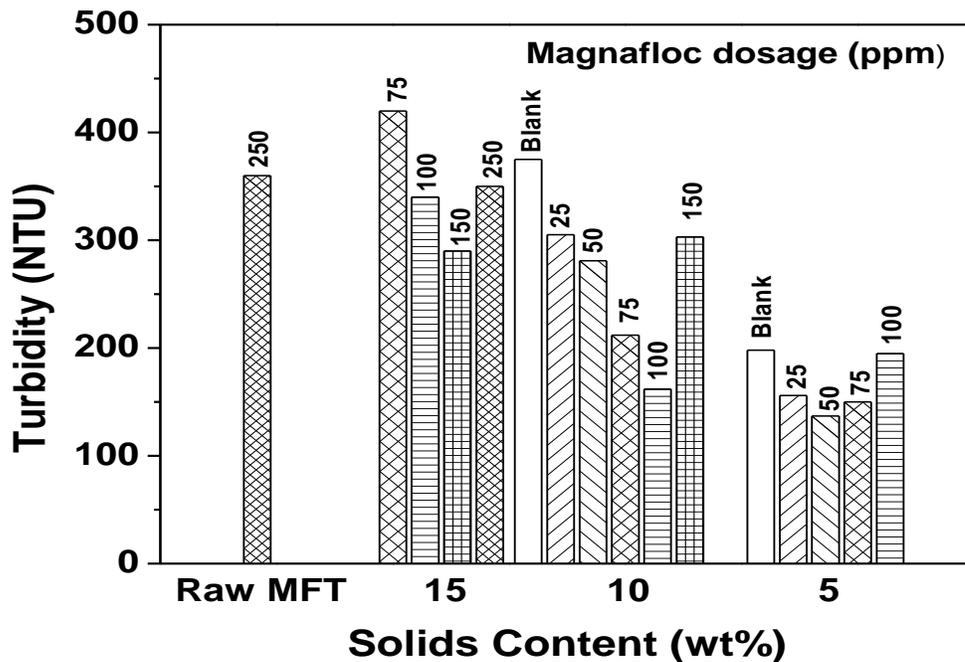
**Figure 3.15** Turbidity of supernatant produced after settling of MFT with MF1011 as flocculant
