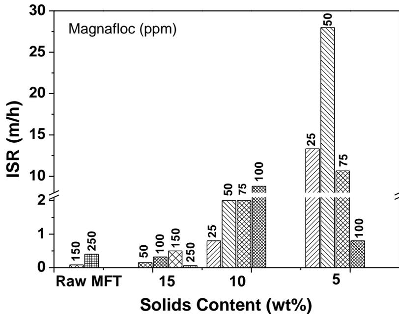
**Figure 3.9** ISRs of MFT diluted to different factors with Magnafloc1011 as flocculant
