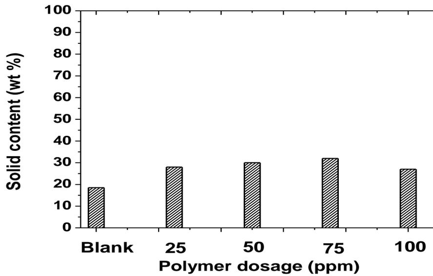
**Figure 3.23** Solid content of the sediment formed by settling of MFT diluted to 10 wt% solids with Al-PAM as flocculant
