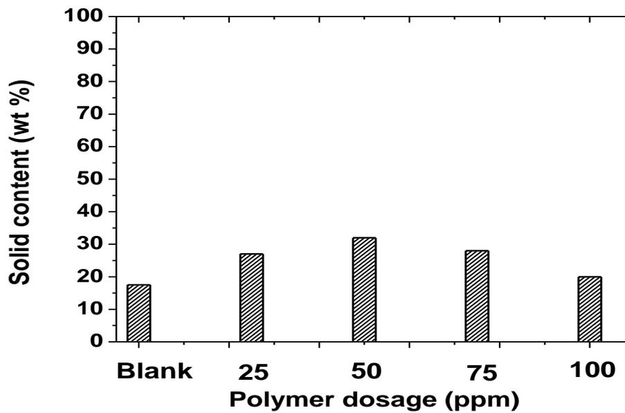
**Figure 3.24** Solid content of the sediment formed by settling of MFT diluted to 5 wt% solids with Al-PAM as flocculant
