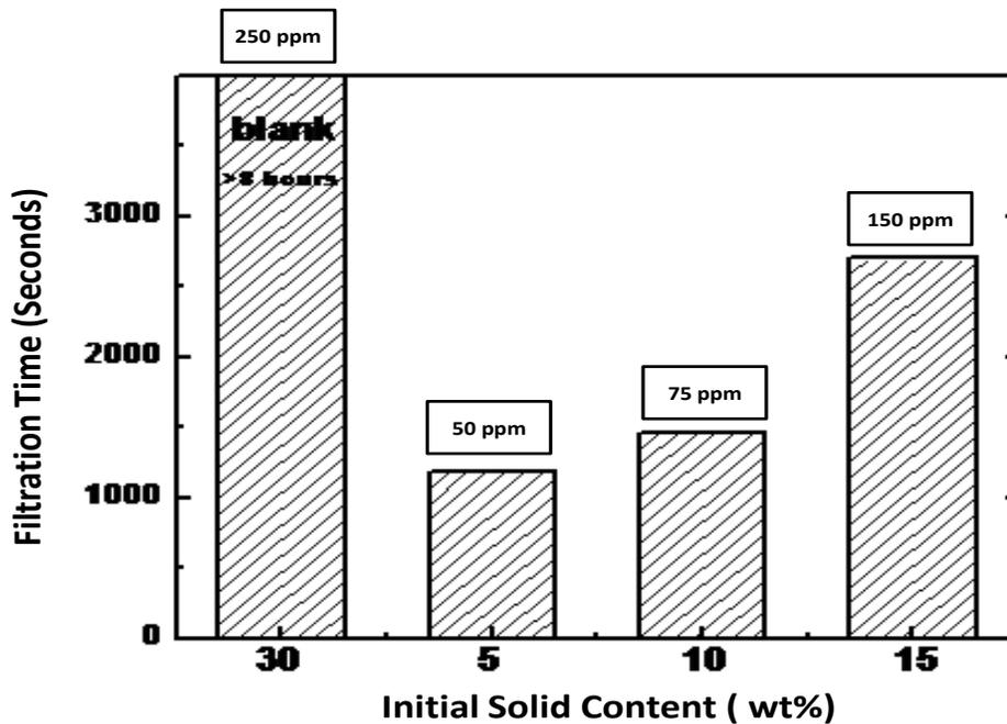
**Figure 3.29** Filtration time of diluted MFT with their respective optimal dosage of Al-PAM to produce a cake of 23 wt% moisture content
