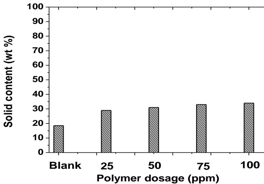
**Figure 3.21** Solid content of the sediment formed by settling of MFT diluted to 10 wt% solids with MF1011 as flocculant
