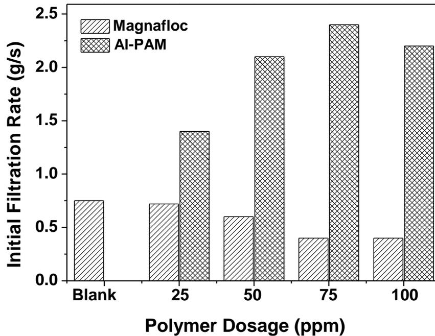
**Figure 3.28** Filtration of MFT diluted to 10 wt% solids with different dosages of MF1011 and Al-PAM
