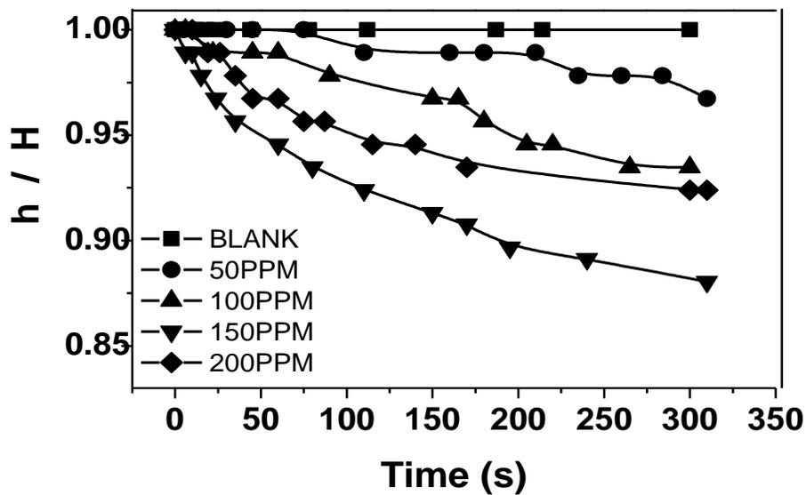
**Figure 3.3** Settling curves of diluted MFT (15 wt% solids) with MF1011 as flocculant
