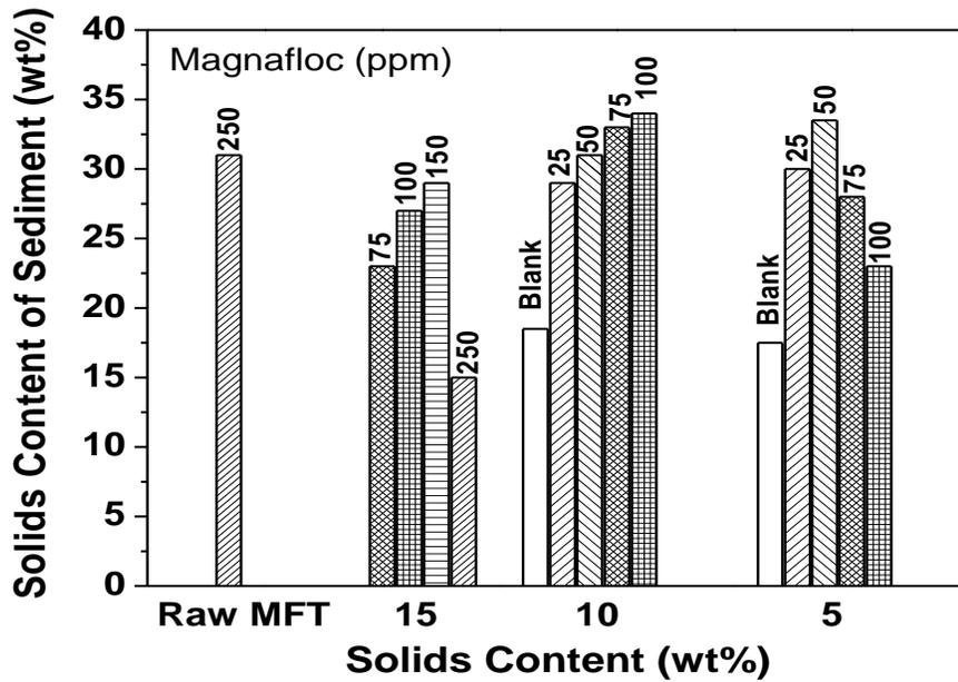
**Figure 3.19** Solid content of sediment after settling of undiluted and diluted MFT with MF1011 as flocculant
