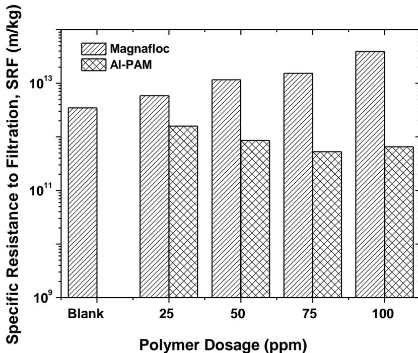
**Figure 3.30** Specific resistance to filtration (SRF) of MFT diluted to 10 wt% solids as a function of Al-PAM dosage
