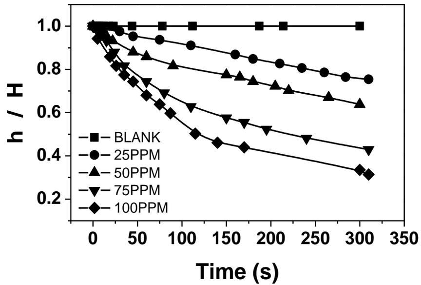
**Figure 3.5** Settling curves of diluted MFT (10 wt% solids) with MF1011 as flocculant
