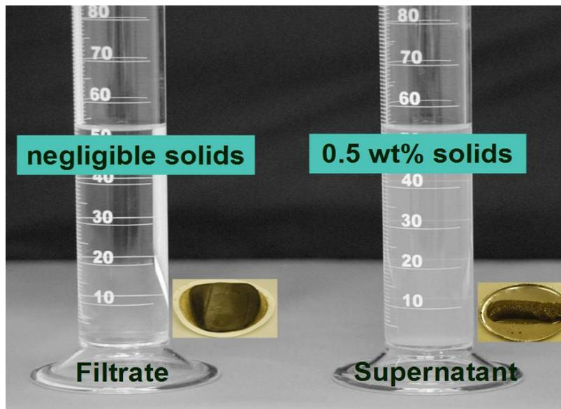
**Figure 3.32** Comparison of release water clarity by thickener and filtration and fluidity of sediments and filter cake (inset)
