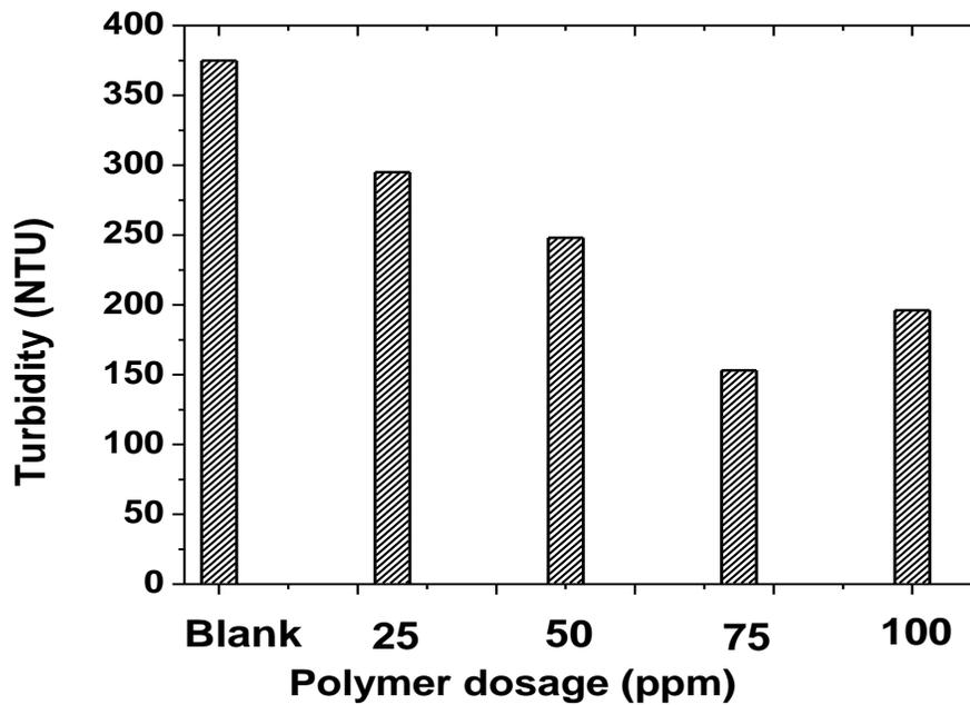
**Figure 3.12** Turbidity of supernatant recovered from MFT diluted to 10 wt% solids with Al-PAM as flocculant
