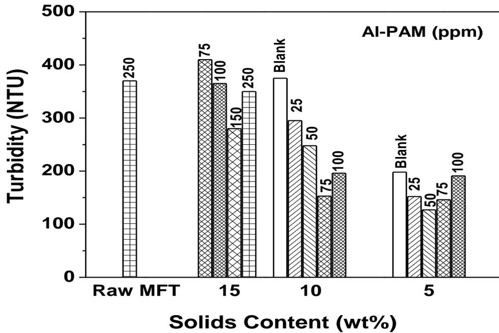
**Figure 3.16** Turbidity of supernatant produced after settling of MFT with Al-PAM as flocculant
