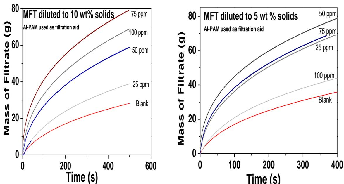
**Figure 3.27** Filtration rate of MFT diluted to 10 wt% and 5 wt% solids with Al-PAM as filtration aid
