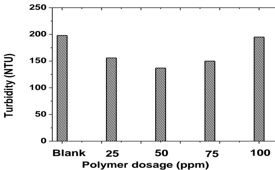
**Figure 3.13** Turbidity of supernatant recovered from MFT diluted to 5 wt% solids with MF1011 as flocculant
