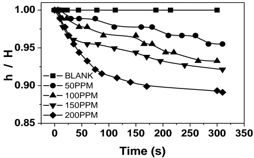
**Figure 3.1** Settling curves of raw MFT (31 wt% solids) with MF1011 as flocculant
