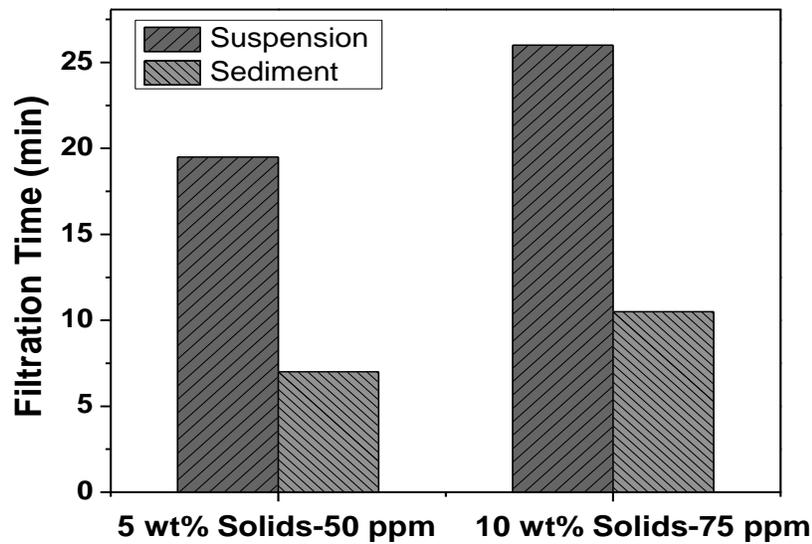
**Figure 3.31** Comparison of filtration time for diluted MFT and corresponding thickened sediments after flocculation at optimal Al-PAM dosage to produce cake (23 wt% moisture)
