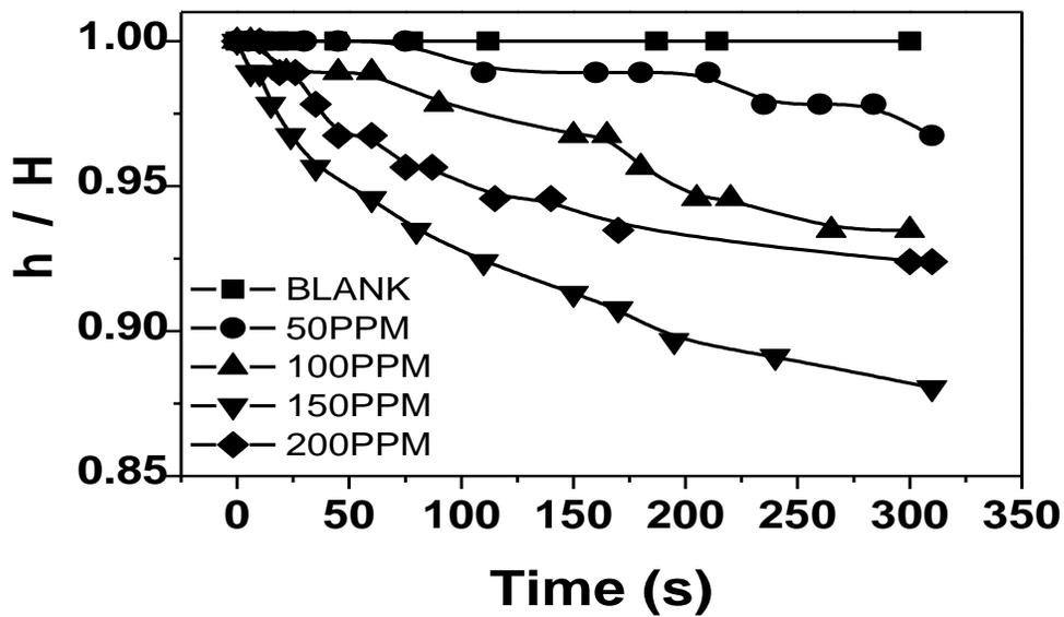
**Figure 3.4** Settling curves of diluted MFT (15 wt% solids) with Al-PAM as flocculant
