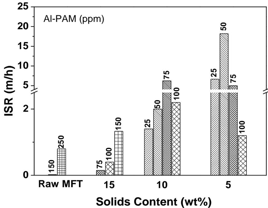
**Figure 3.10** ISRs of MFT diluted to different factors with Al-PAM as flocculant
