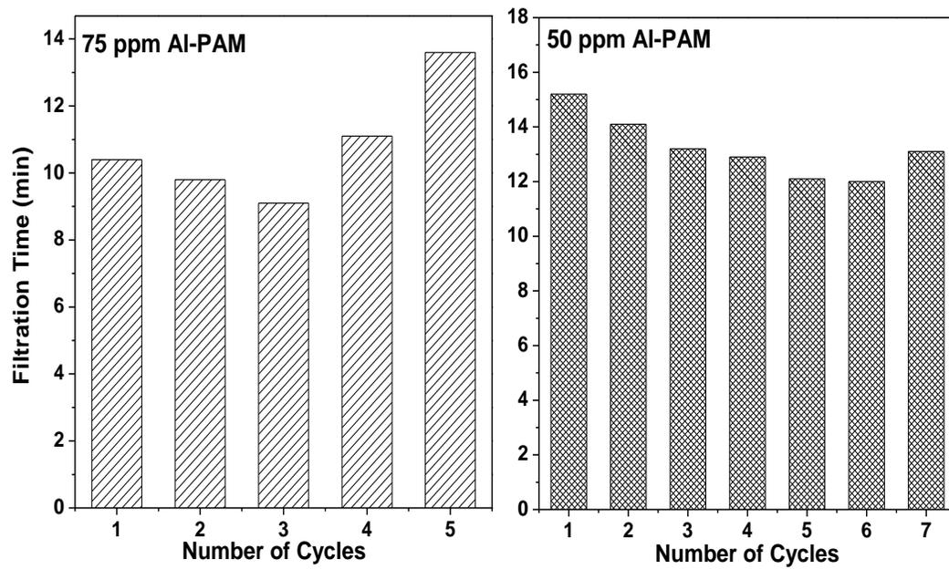
**Figure 3.33** Effect of water recycling on filtration time
