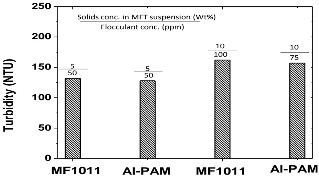
**Figure 3.17** Turbidities of supernatants recovered after sedimentation of diluted MFT with their respective optimum polymer dosages
