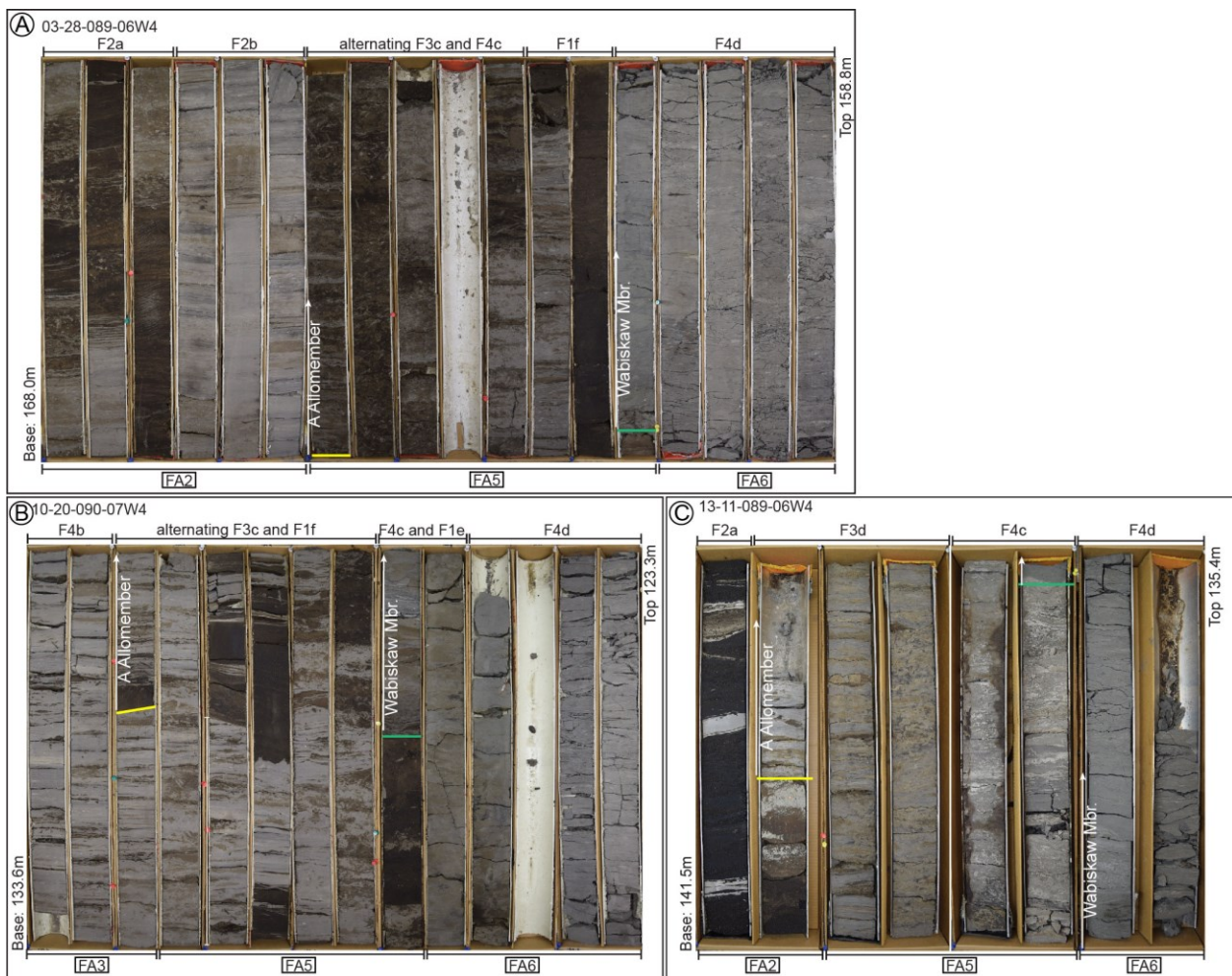
Figure 2.11 Variable core expressions of FA5 brackish-water embayment and FA6 shoreface to offshore in well 03-28-089-06W4, well 10-20-090-07W4, and well 13-11-089-06W4. A) Allomember A showing FA5 brackish-water embayment deposits, consisting of alternating homogeneously bioturbated sandstone and mudstone (F3c) and weakly bioturbated, planar stratified mudstone (F4c). B) Allomember A in well 00-20-090-07W4, consisting of alternating homogeneously bioturbated sandstone and mudstone (F3c) and bioturbated massive sandstone (F1f). Note the sharp contacts between facies. C) Allomember A in well 13-11-089-06W4, consisting of intensely bioturbated sandstone and mudstone (F3d) gradationally overlain by variably bioturbated, planar stratified mudstone (F4c). Green line marks the top of the McMurray Formation and yellow line corresponds to the base of Allomember A.
