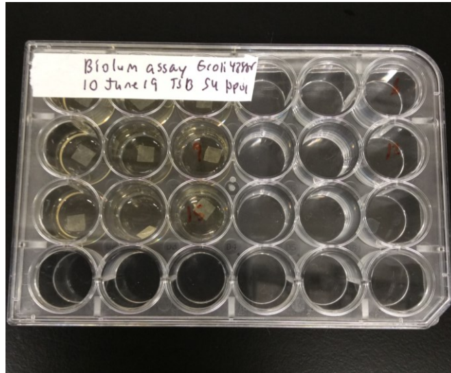
Figure 3.12: A 24-well plate containing phage immobilized PHB substrates and TSB media.
