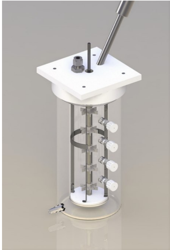
Figure 2-2: Experimental setup for tests of demulsifier performance in bitumen froth. The confined impeller stirred tank (CIST) has 4 side sampling ports and a Teflon lid with two access ports for demulsifier injection (left) and the FBRM probe (right).
