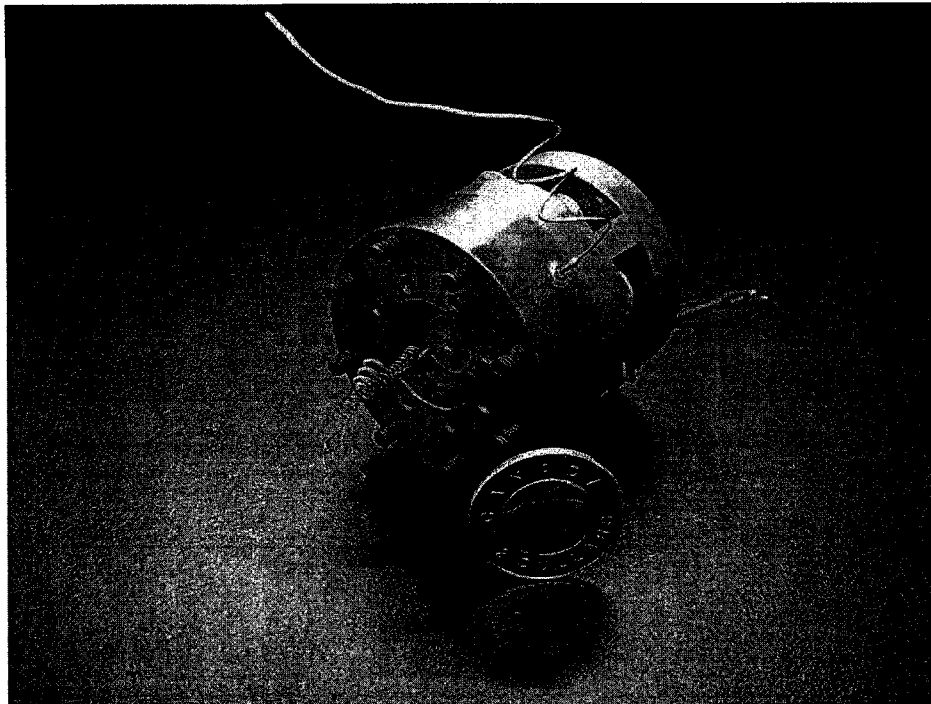
Figure 6.6: Image of the bulk squeezing cell, next to a Canadian twoonie coin for scale.
