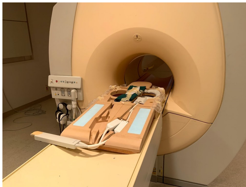
Figure 2.29: Specially designed breast board with Philips Flex-L surface coil.
