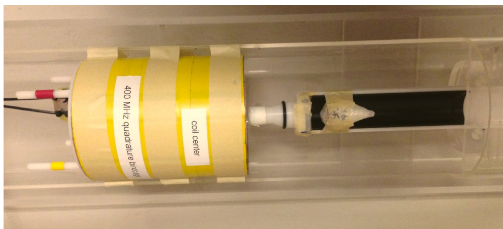
Figure 2.20: 9.4 T Birdcage RF coil with secured phantom. The yellow and red screws are used to tune and match the coil to the load.
