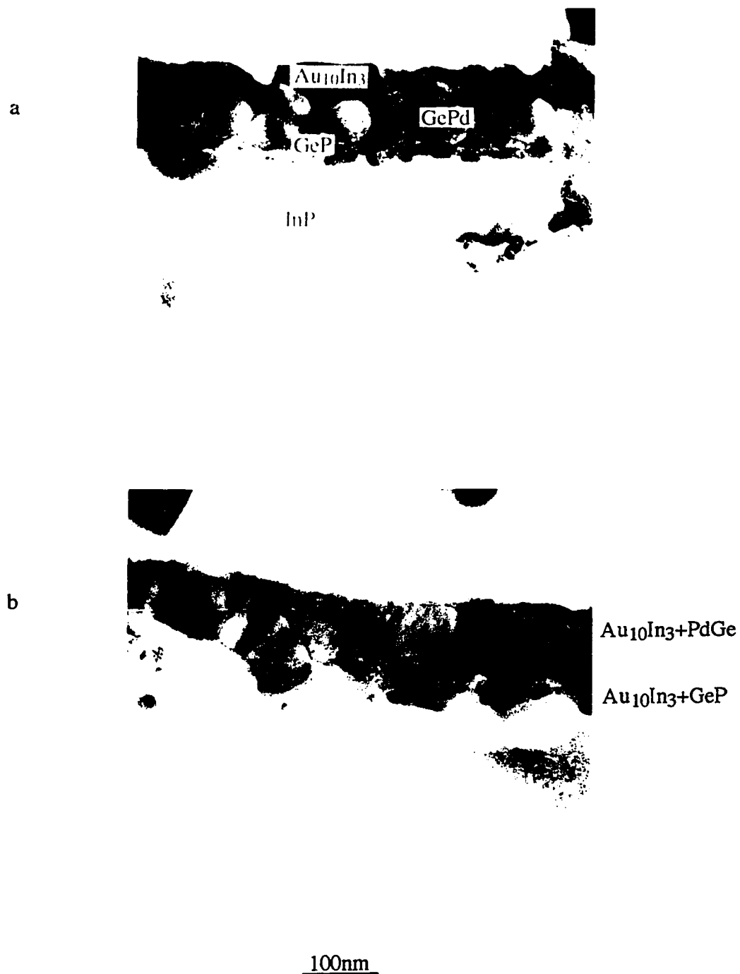
Fig. 7-4 Bright field micrographs of cross section specimens annealed at a) 325°C for 5s and b) 350°C for 180s.
