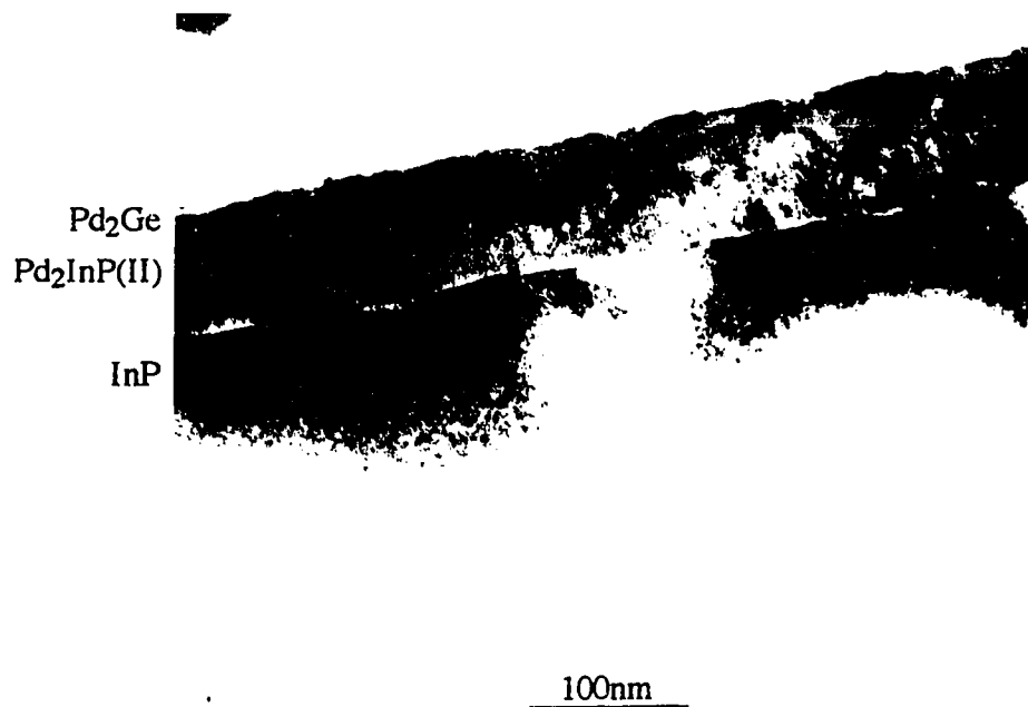
Fig. 7-13a Bright field micrograph of a cross section specimen annealed at 350°C for 20s.
