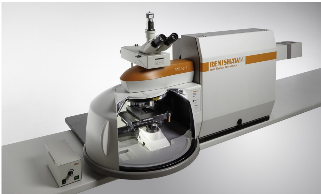
Figure 12: Renishaw InVia™ Raman Microscope ( https://www.renishaw.com/en/invia-confocal-raman-microscope--6260 ) present at the nanoFAB, University of Alberta.
