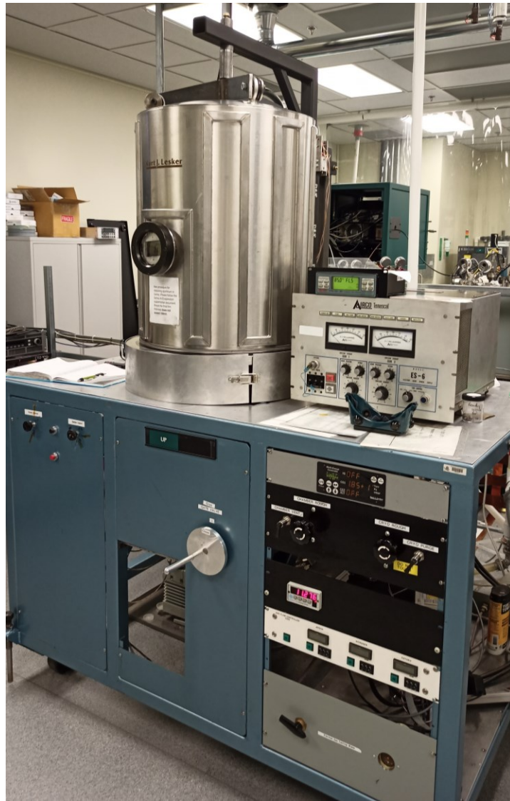
Figure 13: Kurt J. Lesker electron beam evaporator (GOMEZ) ( https://www.lesker.com/ ) present at the nanoFAB, University of Alberta.
