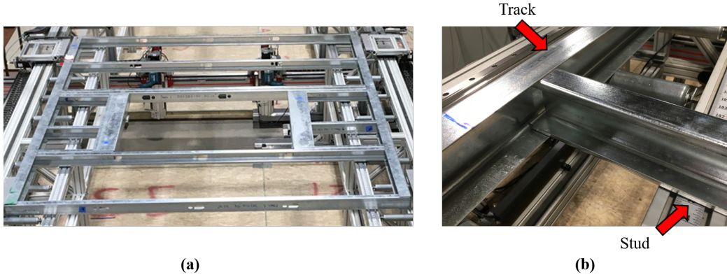
Figure 4.1: (a) Typical steel frame with a door component, and (b) detailed view of a typical intersection. Note that the stud goes inside the track forming 3D intersection.
