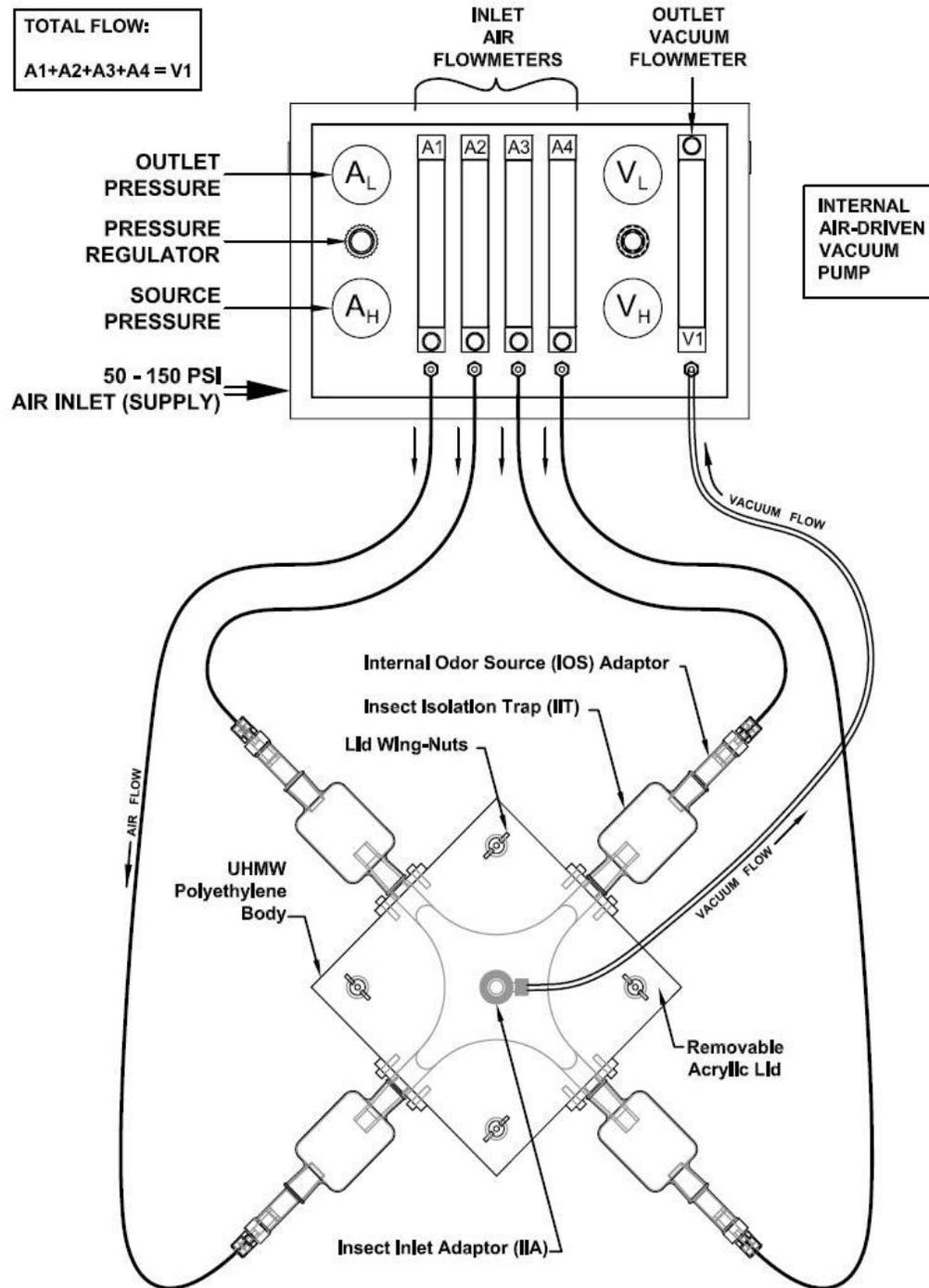
Figure 3.1. System diagram of the four-chambered olfactometer used in olfactory bioassays conducted to test whether olfactory cues associated with the fecal coat of *Oulema melanopus* larvae contribute to host-finding behaviour of *Tetrastichus julis* (Source of schematic: Analytical Research Systems Inc., Gainesville, USA).
