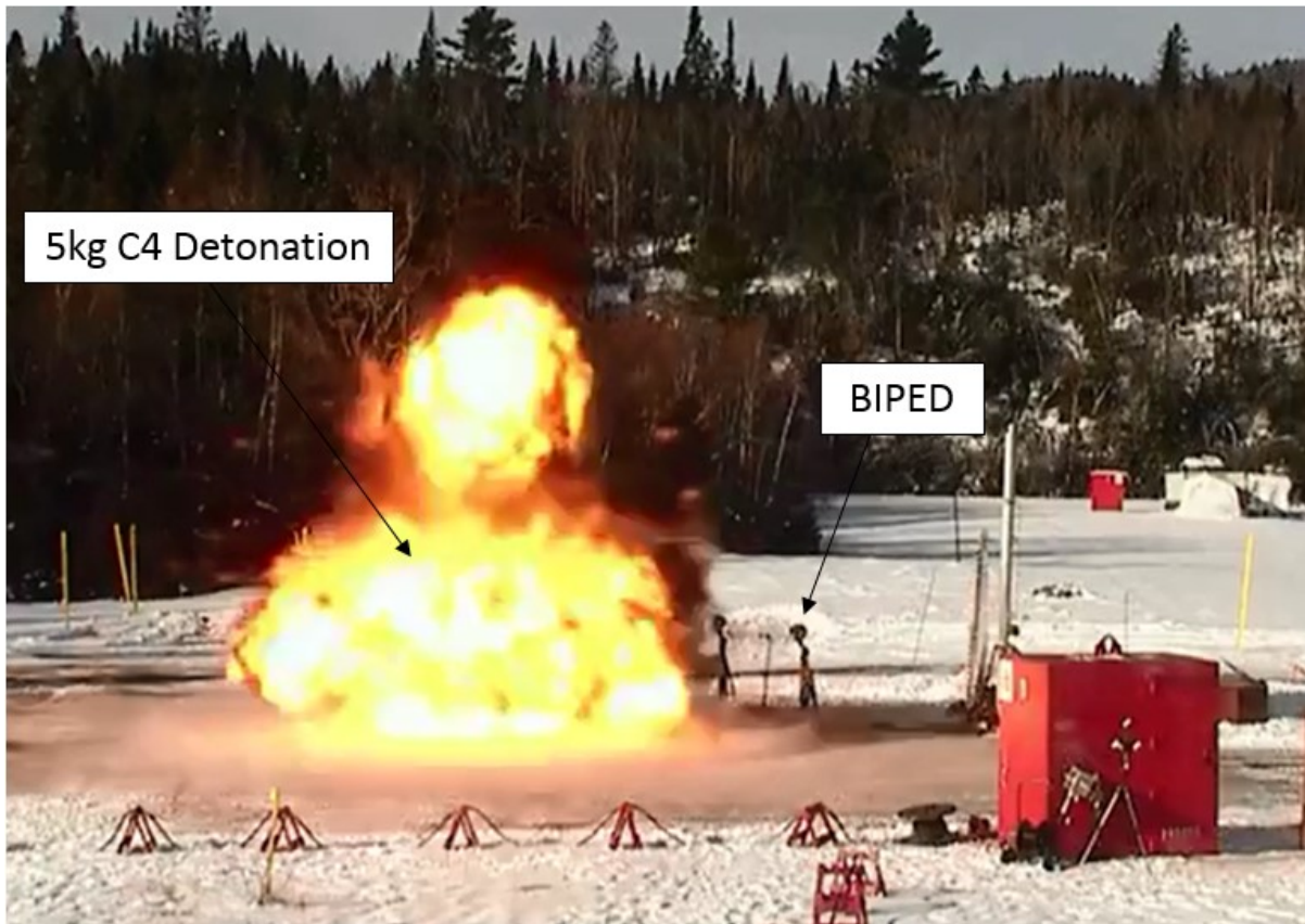
Figure 21: Blast test site showing the resulting fireball from a 5kg C4 detonation and BIPED location during experiments.
