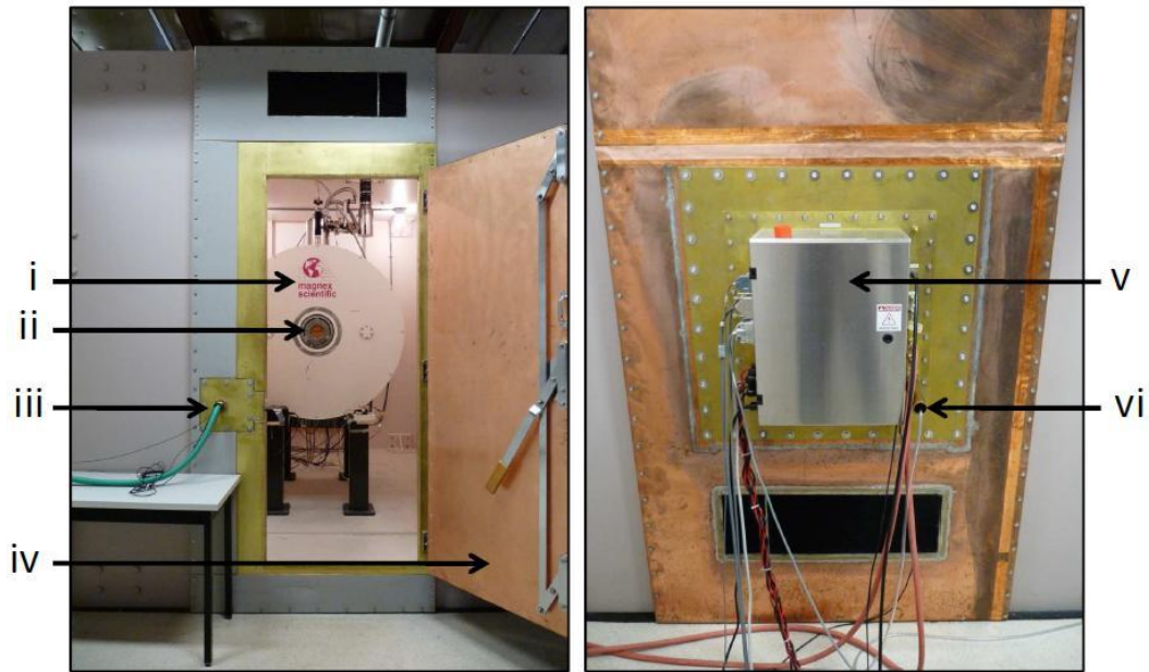
Figure 3.2. Exterior photographs of magnet vault. Front view (left) shows view through vault door including cryostat (i), magnet bore (ii), front wave-guide (iii), and vault door (iv). Rear view shows rear RF filter panel (v) and rear wave guide (vi).
