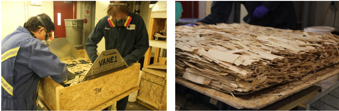
Figure 3.1 Mat formation process: forming box (left), and unconsolidated OSB mat (right)
