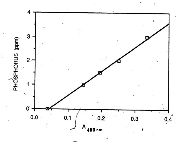
Figure 4.11 Calibration curve for phosphorus determination. Phosphorus was determined spectrophotometrically as a yellow molybdo-vanadate complex, after ashing samples in an oxygen bomb (Yuen and Kelly, 1980).
