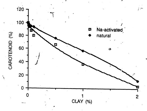
Figure 4.15 Efficiency of Na-activated and natural (Bentonite) clay on carotenoid removal from commercial canola oil. Points on graph represent average of three replicates.
