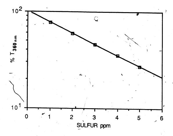
Figure 4.12 Calibration curve for sulfur determination. Sulfur was determined spectrophotometrically as a methylene blue complex with bismuth reagent, after wet digestion of samples in Na-hypobromite (Tabatabai and Bremner, 1970).
