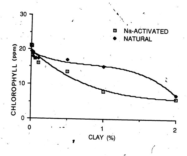
Figure 4.14 Efficiency of Na-activated and natural (Bentonite) clay on chlorophyll removal from commercial canola oil. Points on graph represent average of three replicates.
