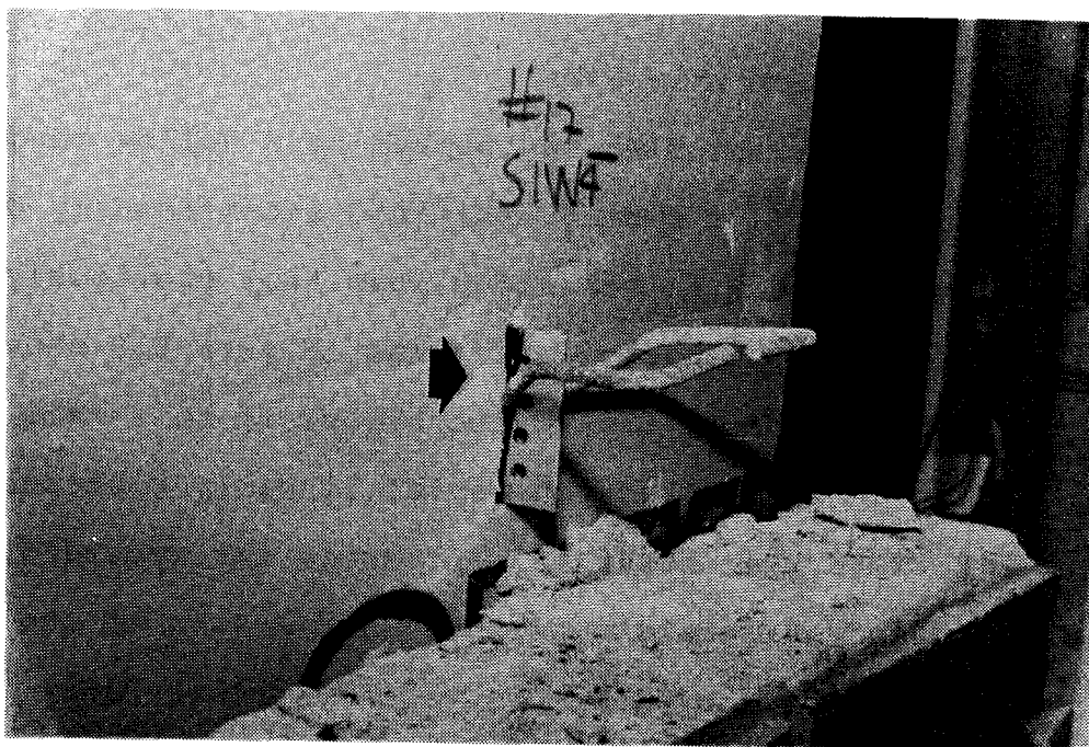
Plate 5.6 Shear Deformation of V Tie Attachment (S1W4)
