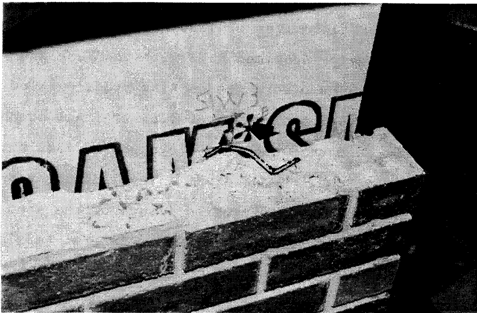
Plate 5.5 Shear Deformation of Rod Tie Attachment (S1W3)
