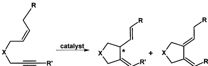
**Equation 12.** Catalyzed enyne cycloisomerization reaction or intramolecular Alder ene reaction. X = NR, O, CR<sub>2</sub>.
