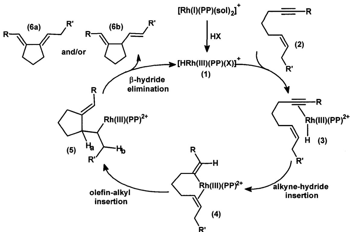
**Scheme 1.** Hydridorhodium mechanism for enyne cycloisomerization by rhodium. The bisphosphine ligand is represented by PP and solvent molecules are represented by sol. X can be  $\text{OAc}^-$ ,  $\text{BF}_4^-$  or other low-coordinating anion.
