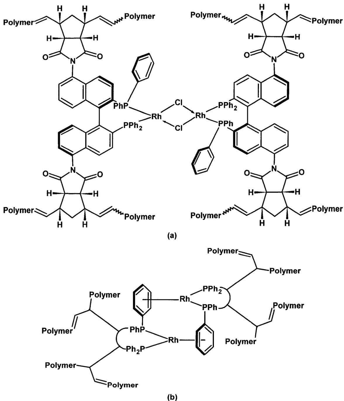
**Figure 29.** Possible forms of the polymerized rhodium catalyst. a) Chloro-bridged dimer prior to addition of  $\text{AgSbF}_6$ . b) Phenyl-bridged dimer prior to the coordination of substrate or following the cycloisomerization completion when no substrate is present. This is a possible resting state of the polymerized catalyst which can potentially be stored like this in the solid state.<sup>121-125</sup>
