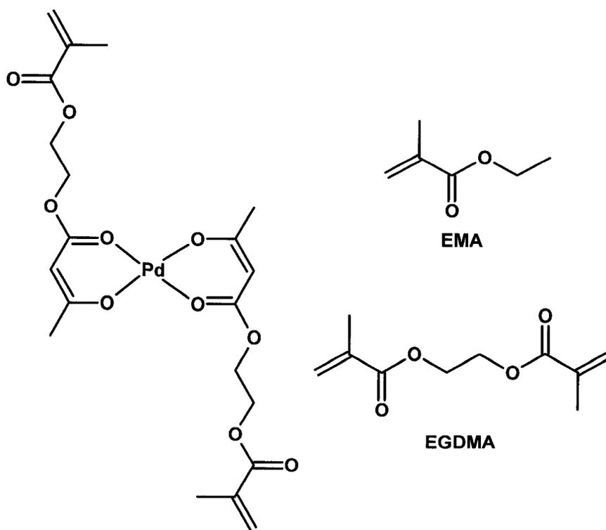
**Figure 7.** Homogeneous palladium catalyst used by Dell'Anna et al. used for the Heck reaction of aryl iodides and various alkenes. EMA and EGDMA were co-polymerized prior to metallation with Pd to form the polymer supported catalyst used.<sup>48</sup>
