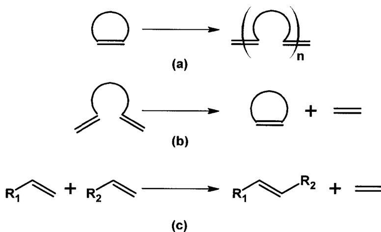
**Figure 3.** Olefin metathesis reactions which can take place. (a) ROMP, (b) RCM and (c) CM.
