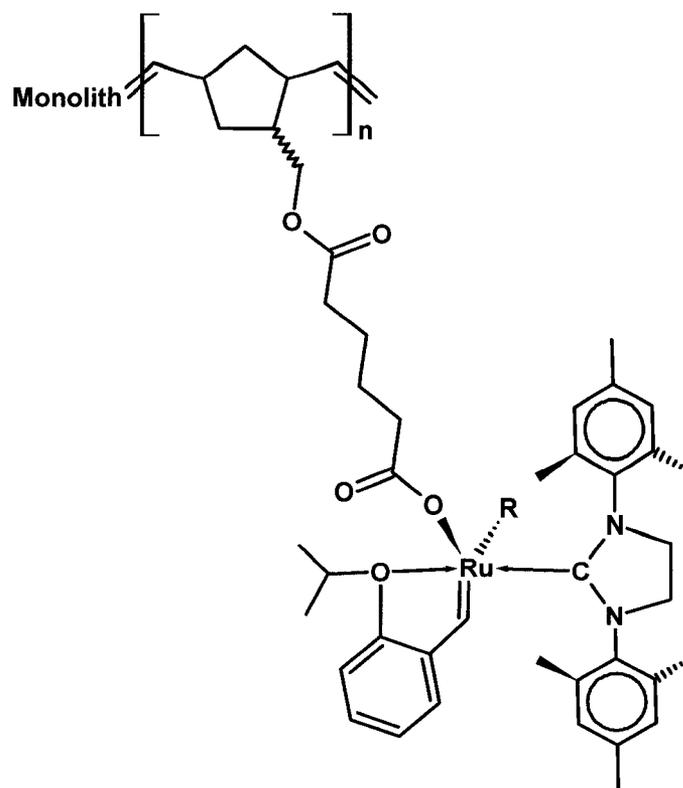
**Figure 5.** The monolith-supported metathesis catalyst used in batch and flow through column reactions by Buchmeiser et al.<sup>26</sup>
