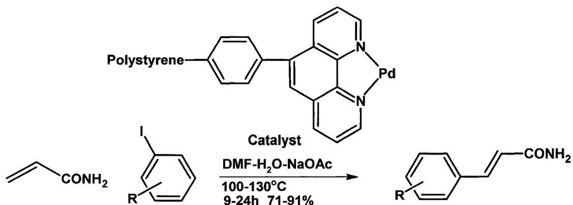
**Equation 6.** Heck reaction of acrylamide with iodobenzenes Zhang et al. using their polystyrene supported palladium catalyst.<sup>47</sup>
