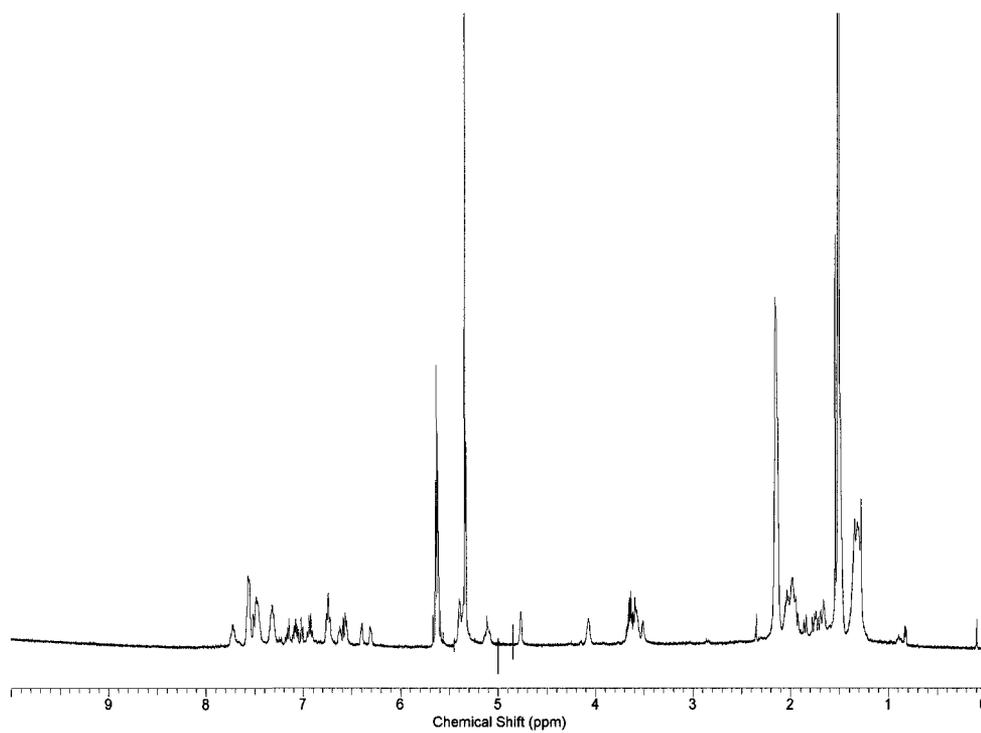
**Figure 27.** <sup>1</sup>H NMR spectrum of  $[\text{Rh}(\text{NBD})(\text{N-BINAP})]\text{BF}_4$  and COE prior to polymerization. See text for analysis.
