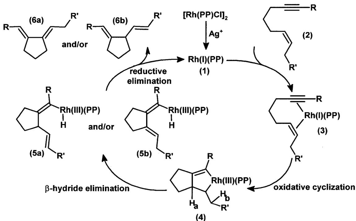
**Scheme 2.** Metallacyclopentene mechanism for enyne cycloisomerization by rhodium proposed by Zhang. The bisphosphine ligand is represented by PP.
