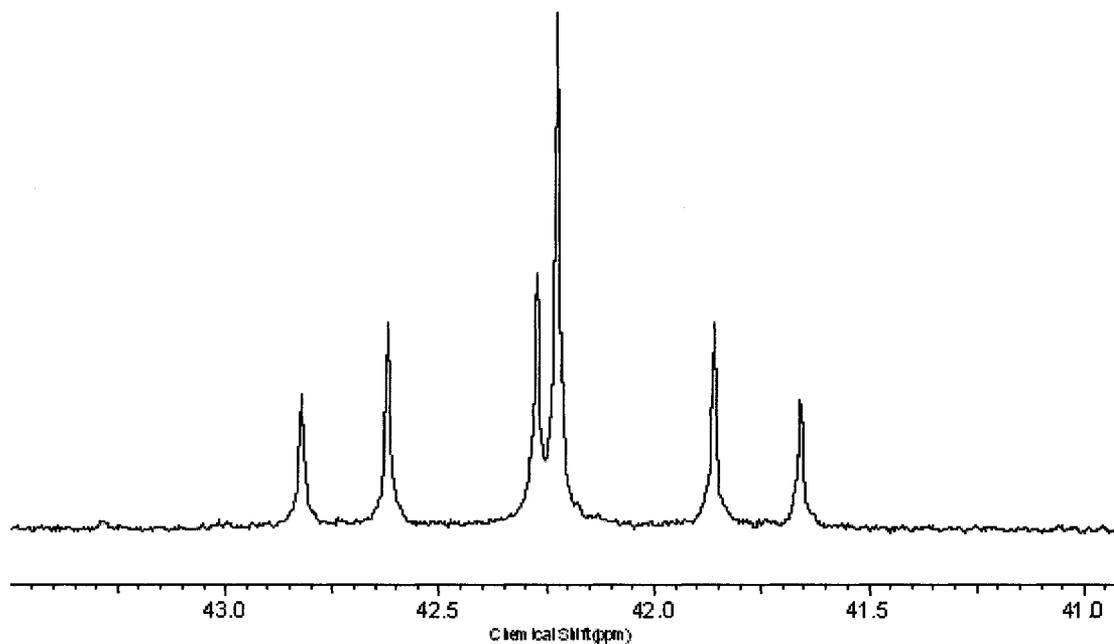
**Figure 22.**  $^{31}\text{P}$  NMR of  $[\text{Ru}(\text{N-Binap})\text{Cl}_2\text{Py}_2]$  at room temperature.<sup>13</sup>
