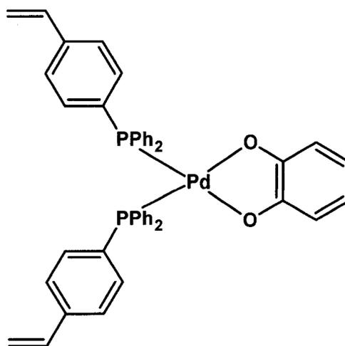
**Figure 10.** Catalyst monomer used by Cammidge et al. for the Suzuki coupling of *p*-bromoanisole and phenyl boronic acid.<sup>52</sup>
