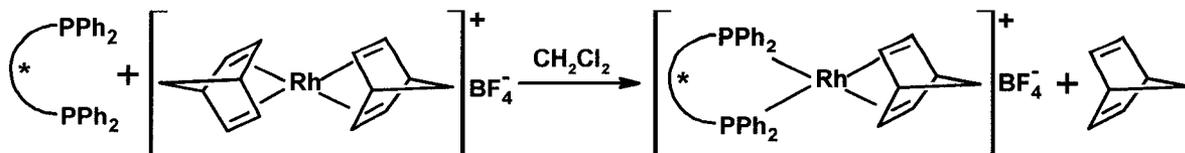
**Equation 19.** Reaction scheme showing the preparation of **10** from  $[\text{Rh}(\text{NBD})_2]\text{BF}_4$  and N-BINAP in  $\text{CH}_2\text{Cl}_2$ .
