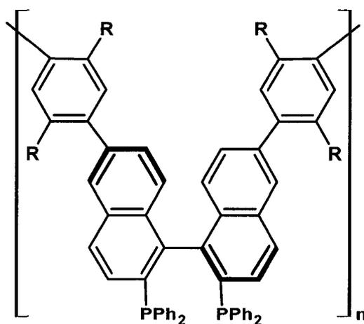
**Figure 12.** (*R*)-BINAP derivative polymerized with 1,4-dibromo-2,5-dialkylbenzene by Pu. The ligand is coupled to rhodium for the reduction of dehydroamino acid derivatives and methylarylketone.<sup>63</sup>
