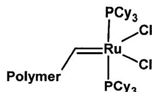
**Figure 4.** Barrett and Braddock's 'boomerang' olefin metathesis catalyst supported by a poly(vinyl polystyrene) backbone.<sup>43-45</sup>
