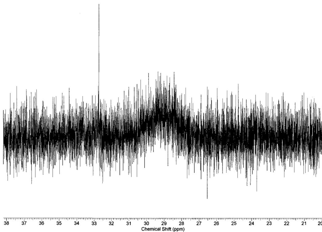
**Figure 26.**  $^{31}\text{P}$  NMR spectrum of co-polymerized  $[\text{Rh}(\text{NBD})(\text{N-BINAP})]\text{BF}_4$  with COE. The peak at 32.6 ppm is 2<sup>nd</sup> Generation Grubbs' Catalyst used for the ROMP reaction. See text for analysis.
