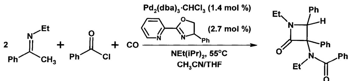
**Equation 2.** One of Arndtsen's palladium-catalyzed  $\beta$ -lactam synthesis from imines, acid chloride and carbon monoxide.<sup>15</sup> dba = dibenzylideneacetone
