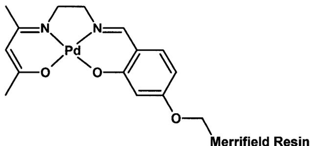
**Figure 11.** Merrifield resin-supported palladium catalyst used by Phan et al. in the Suzuki coupling of heteroaryl bromides and phenylboronic acid.<sup>53</sup>
