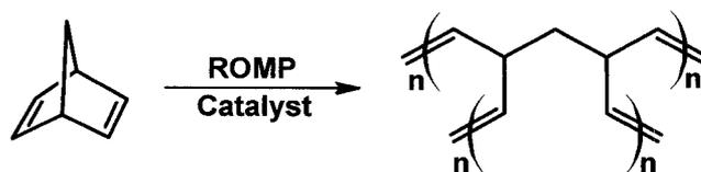
**Equation 20.** ROMP using NBD results in a highly crosslinked, unsaturated polymer.
