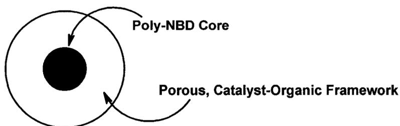
**Figure 29.** The insoluble NBD core is first synthesized followed by the growth of the porous catalyst-organic framework directly grafted onto the NBD core.
