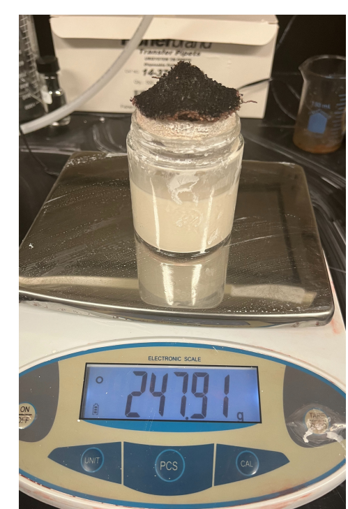
Fig. 3 Mass reading of solar evaporator system
