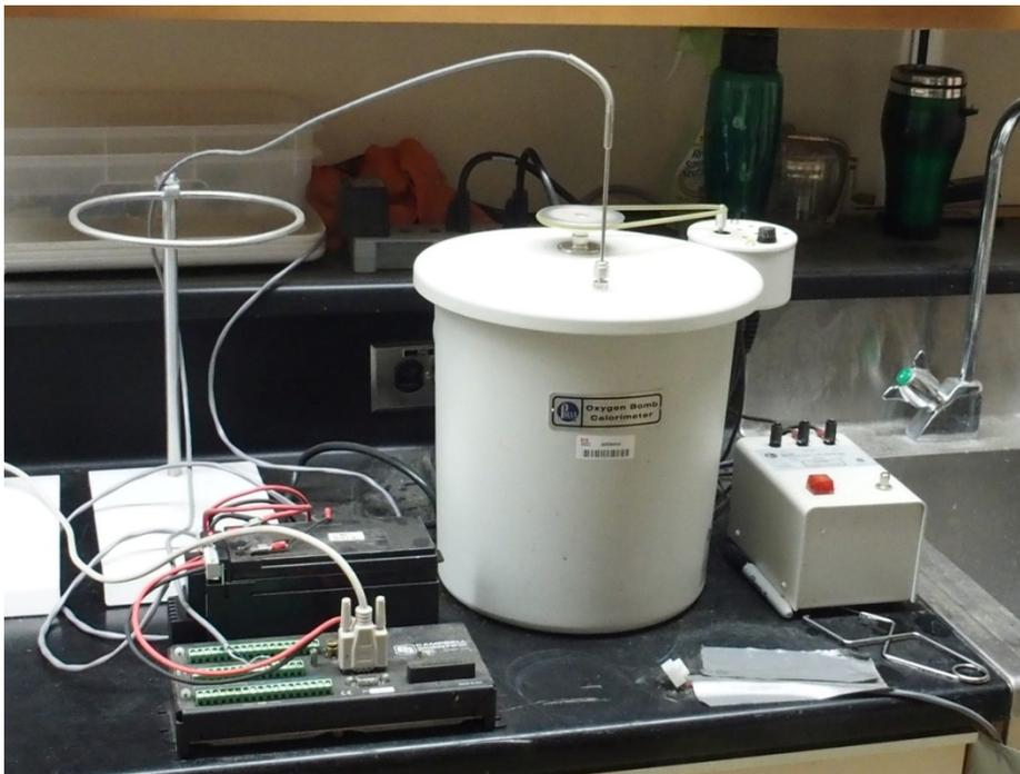
**Figure 2.11** Electrical contacts for ignition of the tested sample are connected (top image); Parr model 1341 Plain Jacket calorimeter ready for the test (bottom image).
