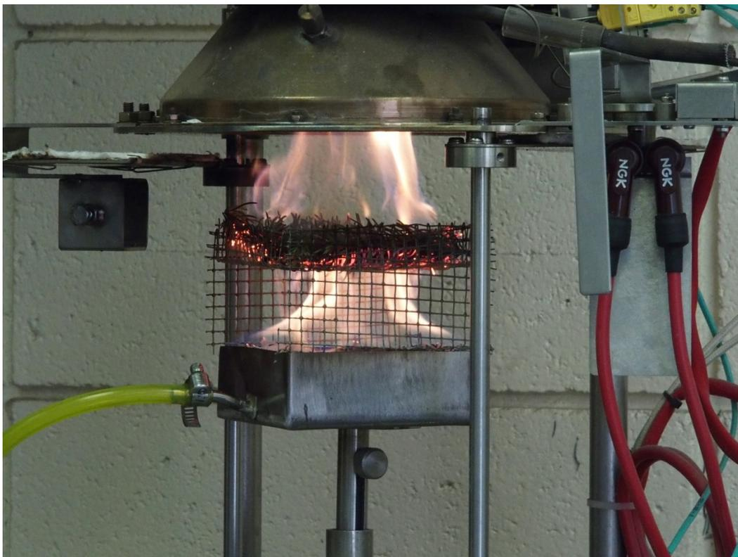
**Figure 4.1** Live fuel burning within the methane flame at several seconds after ignition: new shoots (top image) and 1-year shoots (bottom image)
