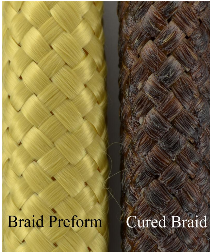
Figure 5.4 – A braid before and after matrix application and curing.
