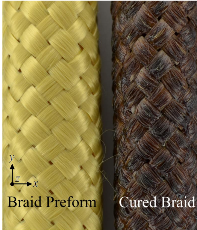
Figure 4.3 – A braided preform and cured braid with the coordinate system convention.
