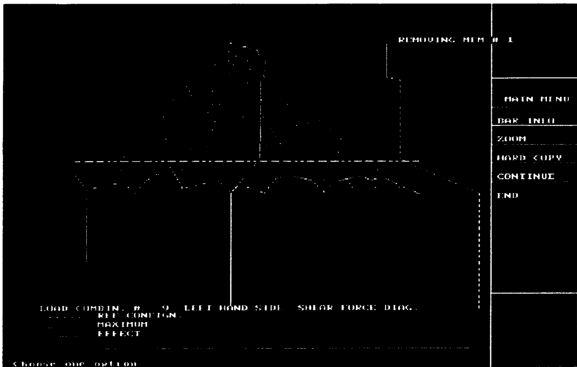
(c) Shear Force Diagram
