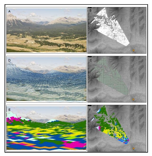
**Figure 3.7**. Procedure for raster analysis of oblique images using the WSL Monoplotting Tool. A) Image to be analyzed, B) Viewshed of image after georeferencing to identify photo origin, C) 100mX100m fishnet grid intersection with the viewshed, D) oblique perspective of fishnet grid overlain on image, E) classified vegetation on image F) orthogonal transformation and spatially referenced classified grid cells.2 column image.
