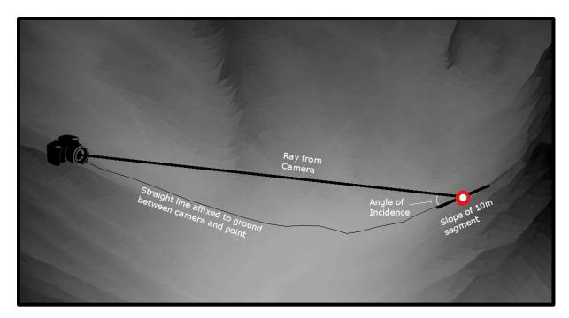
**Figure 3.6**: The angle of viewing incidence between the ray from the camera  $(r_P)$ , and the slope of a 10m line segment from a line between the camera and point *P* affixed to the ground. Lower angles of incidence increase the 3D distance between *P* and *P'*.
