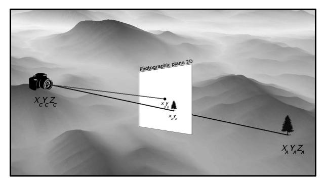
**Figure 3.2**: The collinearity condition as illustrated by the relationship between the camera, and an object with pixel coordinates  $x_ay_a$  in the 2D photographic plane, its real world 3D coordinates  $X_AY_AZ_A$ .  $X_CY_CZ_C$  indicates the location of the camera position in 3D space.
