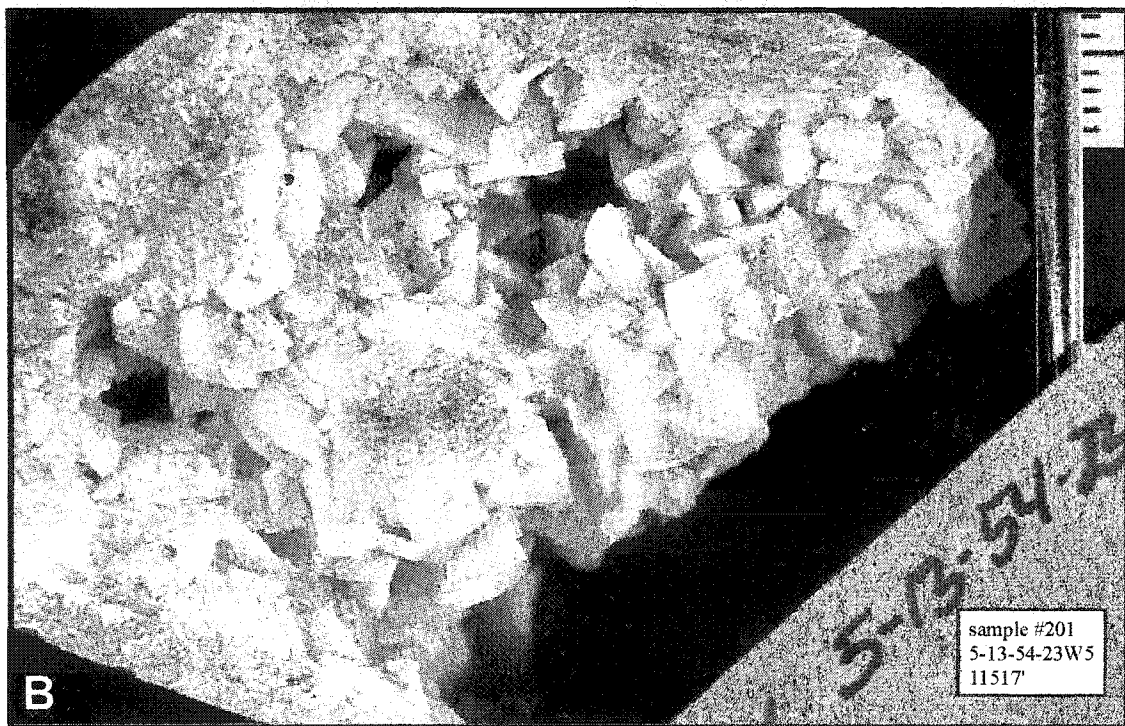
Figure 4.19: A) shows saddle dolomite crystals(SD) in a vug that are covered by solid bitumen and postdated by late blocky calcite spar (CC). B) depicts slightly larger saddle dolomite cements, that are covered with elemental sulfur, indicating that the saddle dolomite formed during TSR.
