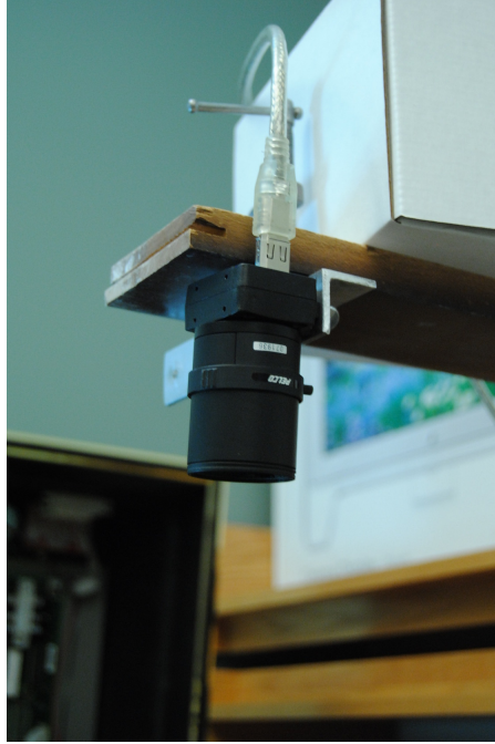
Figure 3.3: A Point Gray FFMV-03M2C camera with a PELCO lens suspended over a pinball machine.
