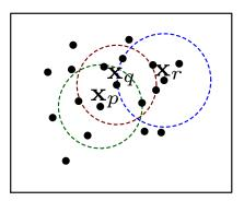
Figure 3.3:  $\mathbf{x}_p$  and  $\mathbf{x}_r$  are density-connected via  $X_q$ .
