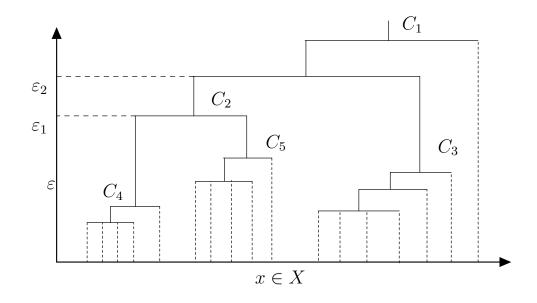
Figure 3.6: Dendrogram for a sample dataset: HDBSCAN\* hierarchy for a sample dataset for minClSize = minPts = 4. Thinner dashed lines denote noise.
