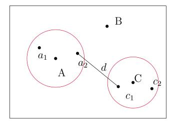
Figure 5.3: Role of Threshold Distance : Consider cluster centers A,B and C sampled from the origin. When cluster A splits into two child clusters  $a_1$  and  $a_2$  and C splits into child clusters  $c_1$  and  $c_2$ , there is a minimum distance that must be maintained between the child clusters of A and C. This is the threshold distance, d.
