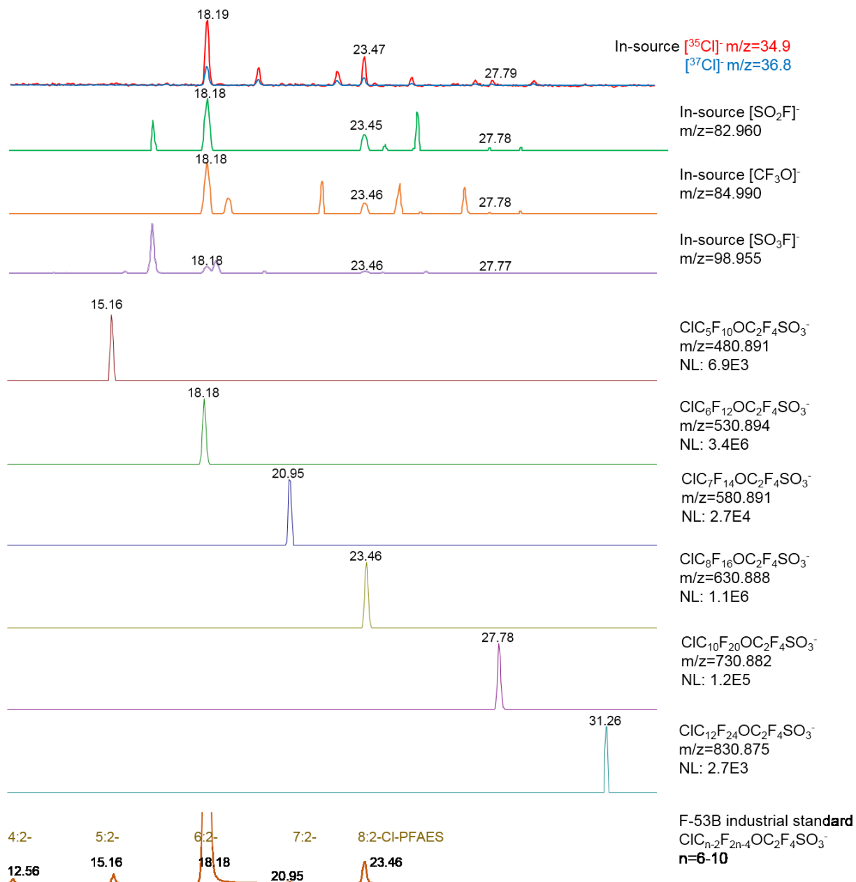
Figure 4-4.1. Extracted ion chromatograms of [Cl] - , [SO 2 F] - , [COF 3 ] - and [SO 3 F] - in-source fragments, and Class 2 x:2 Cl-PFAES (C 1 C n-2 F 2n-4 OC 2 F 4 SO 3 - ) molecular ions detected in pooled common carp liver from the Yangtze River, and of x:2 Cl-PFAESs in F-53B industrial standard.
