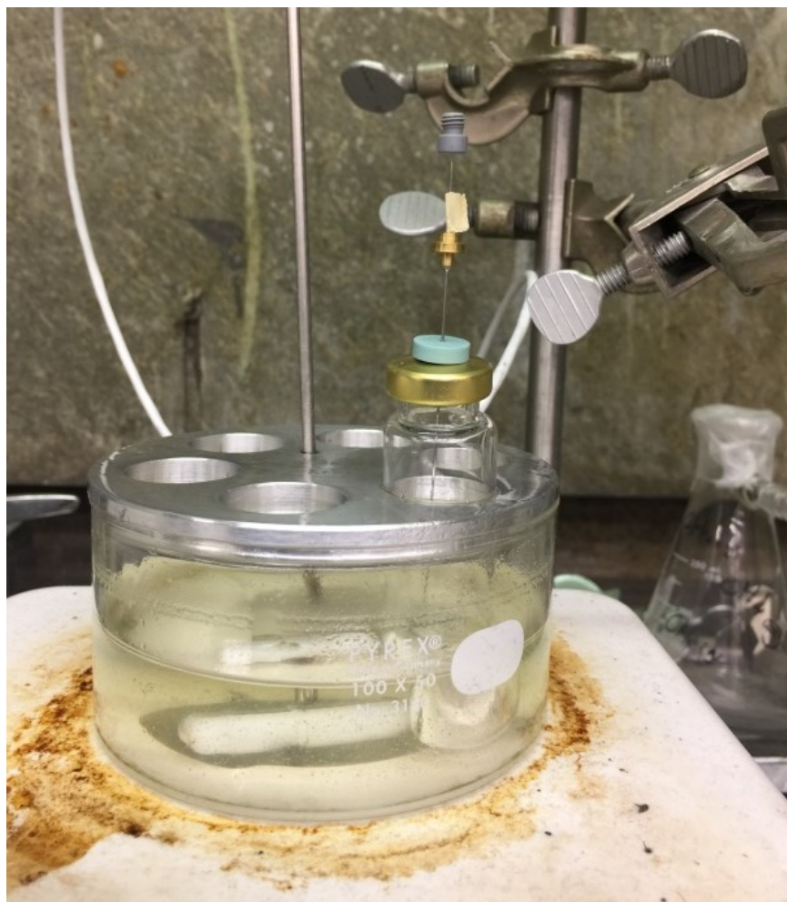
Figure 3.6 Extraction of volatiles from fabric samples in a vial immersed in oil-bath using SPME fibre
