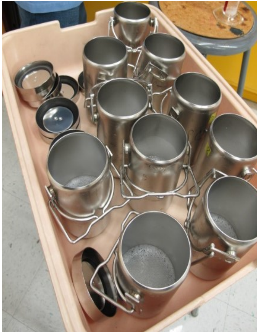
Figure 3.3 Canisters filled with wash solution and steel balls
