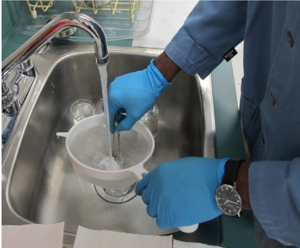
Figure 3.4 Rinsing of fabric samples directly from tap water
