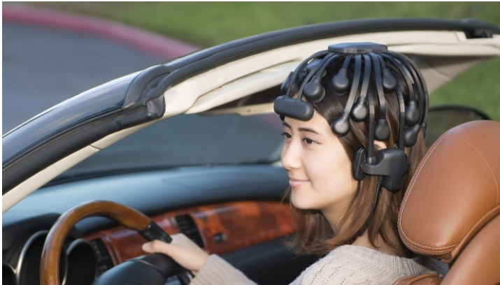
Figure 2.11 Cognionics Quick-20 Dry EEG Headset used by RH Steven's work. Copyright by the Cognionics.
