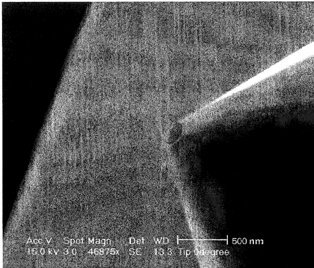
Figure 4.13: The actual aperture formed after the Cr/Ag deposition is revealed in this SEM image. The diameter is determined to be on the order of 200 nm, although aperture size can be tailored by varying the etching time in BOE prior to the Cr/Ag deposition.
