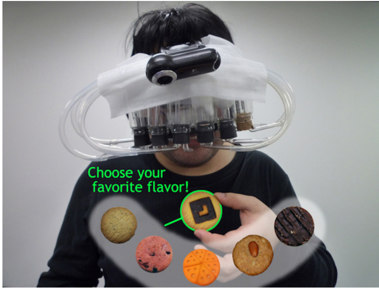
Figure 36: Narumi et al.'s taste simulation system
