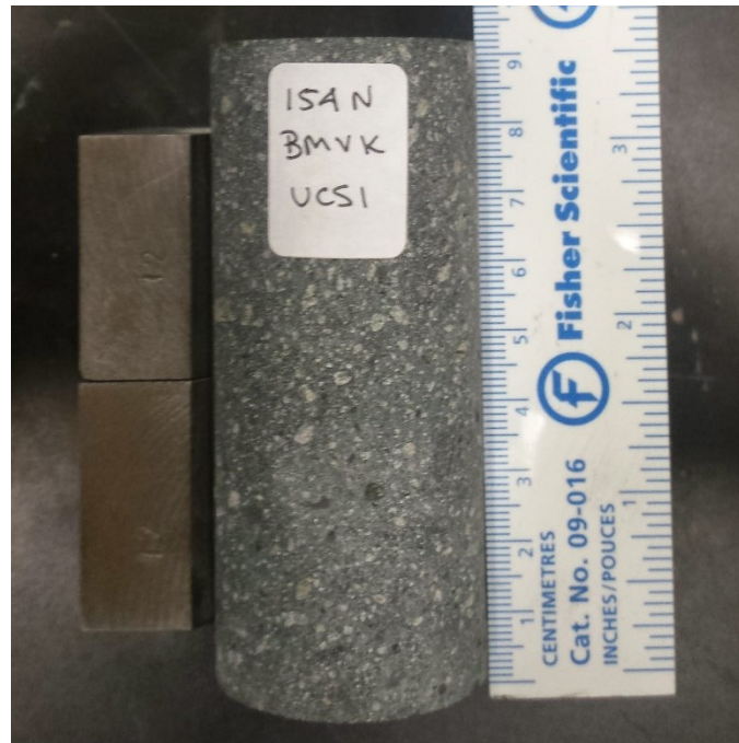
Figure 4.6: Finished sample ready for testing (38mm diameter)
