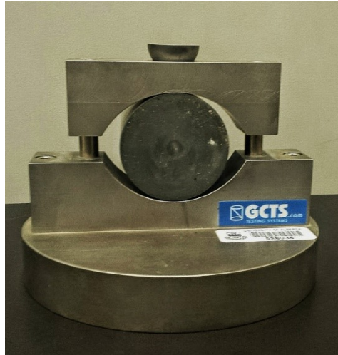
Figure 4.1: Brazilian tensile strength test equipment
