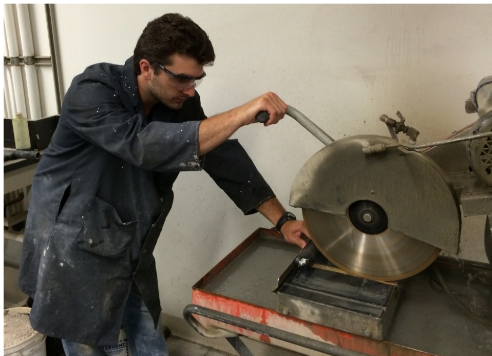
Figure 4.5: Trimming samples with wet saw
