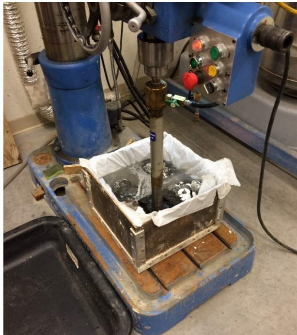
Figure 4.4: Coring of bulk rocks samples
