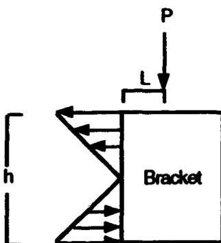
**Free body diagram of a bracket being tested with the Instron Testing Machine (viewed from the mesial aspect).**
