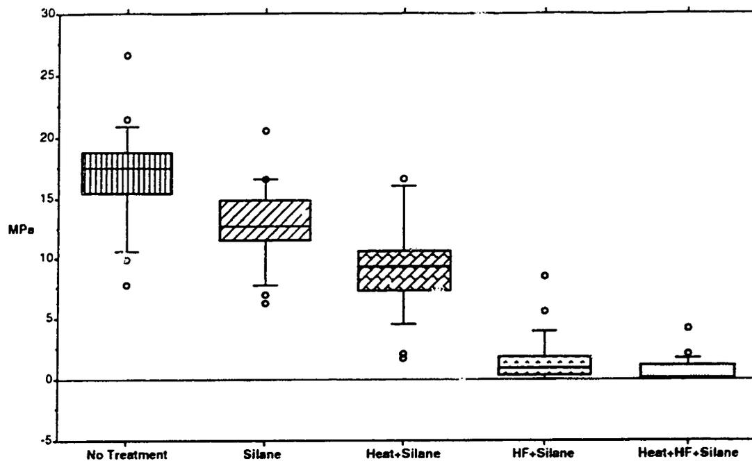
**Figure III. Boxplots of Shear/Peel Bond Strengths (MPa)**
