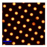
Figure G.4: Confocal reflection image of Al deposits.
