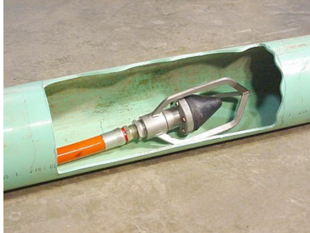
Figure 2.8: The Placement of Nozzle inside a Pipe (Town of Amherst, 2008)
