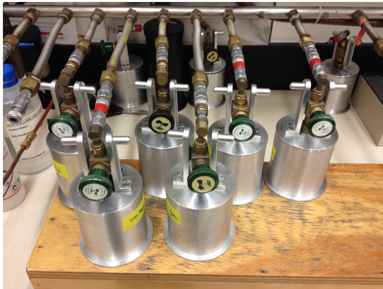
Figure 9: In vitro cell experimental setup: Air tight culture chambers attached to degassing system (vacuum and nitrogen gas supply) to induce hypoxic conditions in these chambers.
