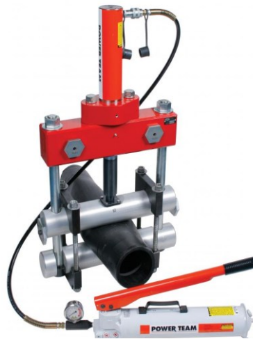
Figure 1-1 Commercial squeeze-off tool for PE pipe [14]
