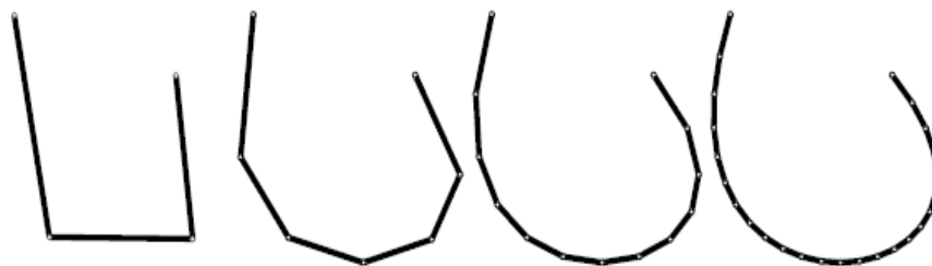
FIGURE 1.1: Example of an interpolatory subdivision scheme for curves in the plane. Initial points remain unchanged while additional points are added by rules related to an interpolatory mask.
