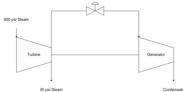
Figure 2.2: Process Flow Diagram of a Turbine Generator
