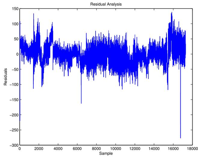
Figure C.19: Model 3 Using 35 psi Steam and Condensate Flow Rates as Input Variables
