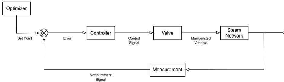
Figure 2.16: Block Diagram of the Optimizer and the Control System
