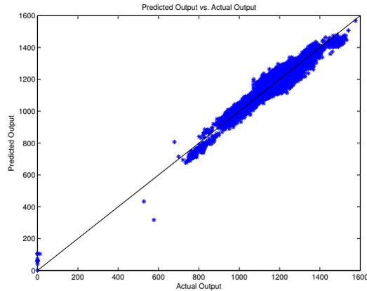
Figure 2.4: Predicted Output vs. Actual Output for Turbine Generator 1 Model
