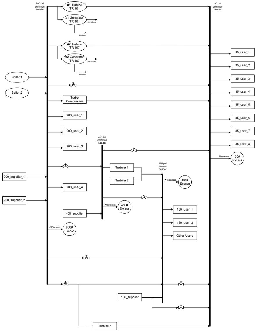
Figure 2.1: Process Flow Diagram of the Utilities Plant
