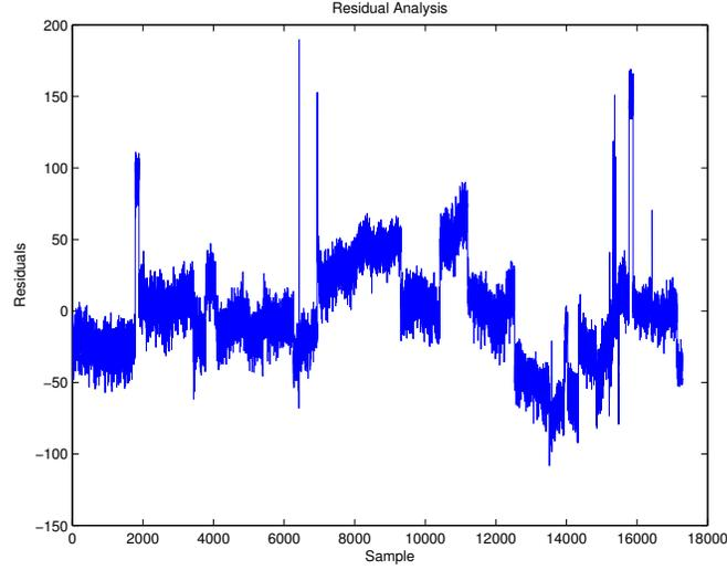
Figure C.57: Model 1 Using 900 psi Steam and 35 psi Steam Flow Rates as Input Variables
