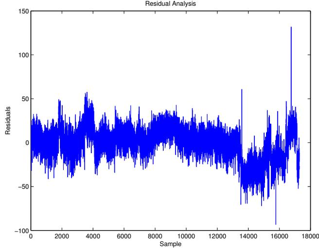
Figure C.39: Model 3 Using 35 psi Steam and Condensate Flow Rates as Input Variables
