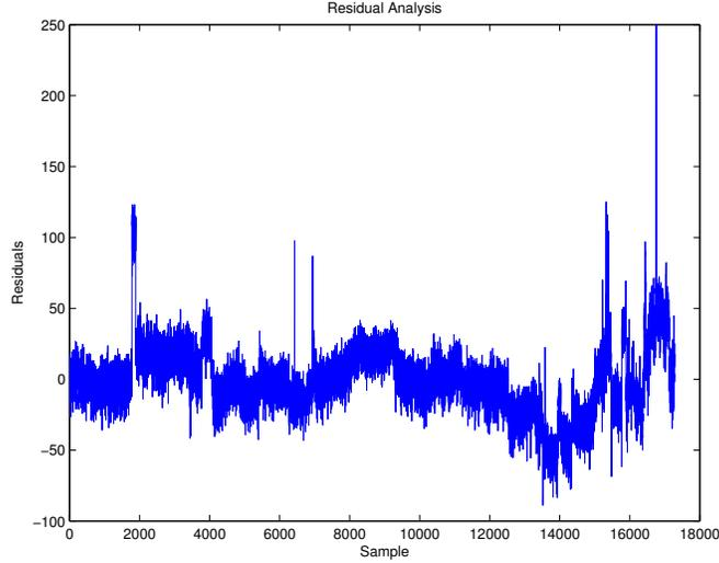
Figure C.42: Model 2 Using 35 psi Steam and Condensate Flow Rates as Input Variables
