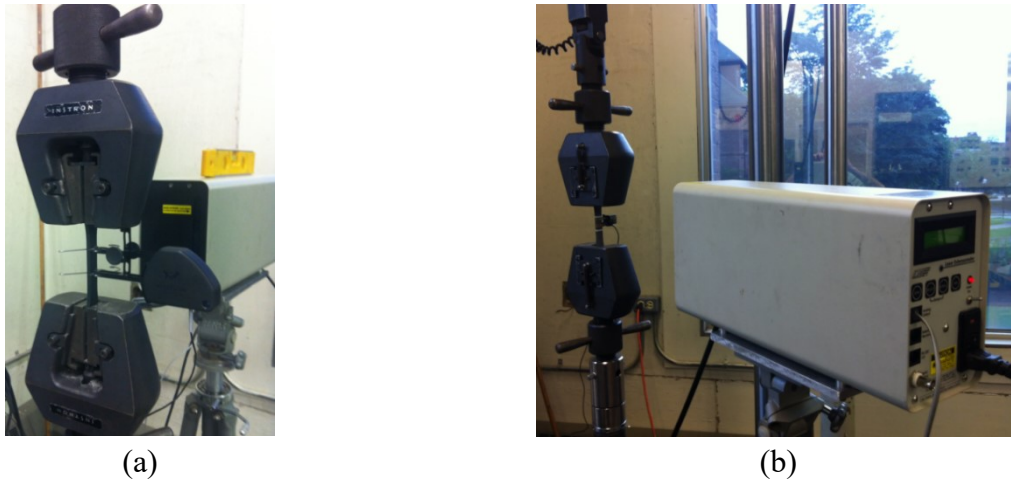
Figure 3. 2 Experimental setup for the (a) static; (b) quasi-static and higher loading rate tests.
