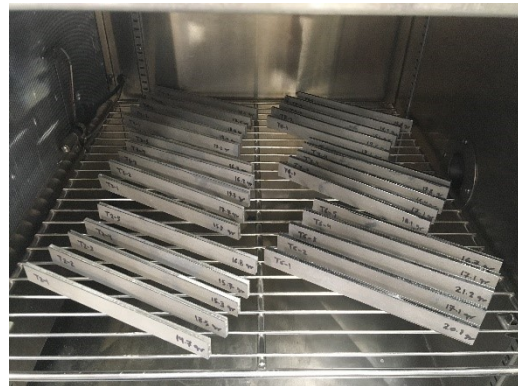
Figure 6.1 (a) Typical heating/cooling cycle, and (b) specimens in the environmental chamber.
