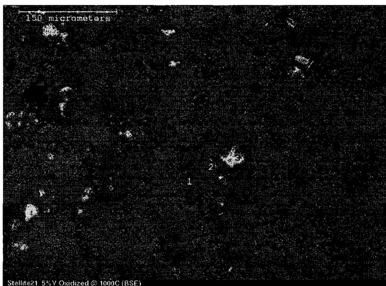
Figure 7.18: SEM image of the oxide scale developed on 5% yttrium-containing sample showing the locations of the EDS point analysis.
