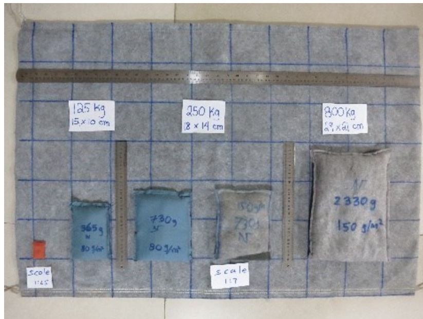
Figure 2-4: Four different sized geobags used in the physical model experiment (the orange bag was used in the 2010 NHC study)
