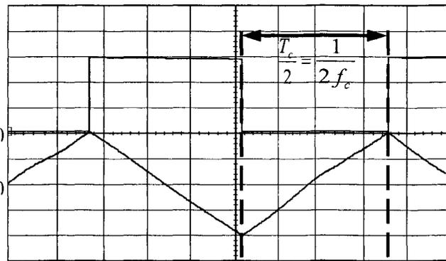
(b) Sawtooth carrier generator waveforms:  $v_{sq}$  and  $v_{saw}$
