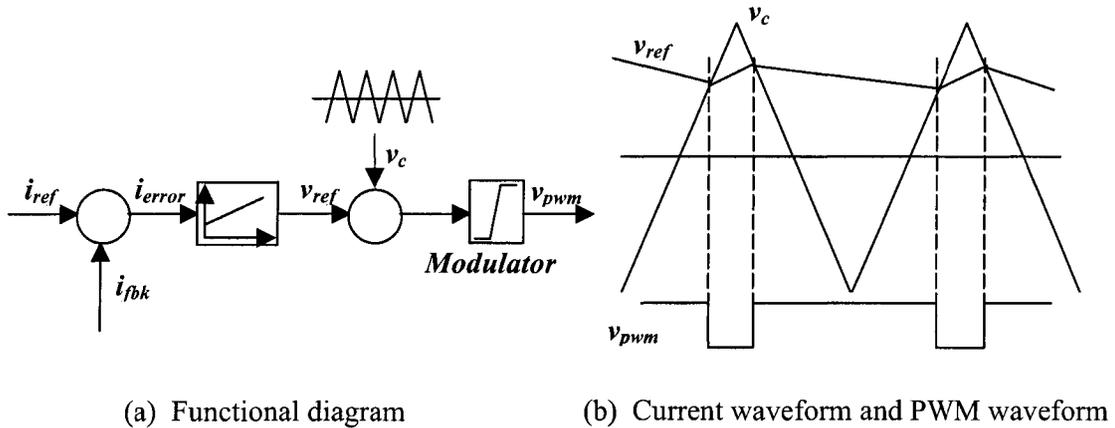
Fig. 2.2 Carrier-based current control scheme
