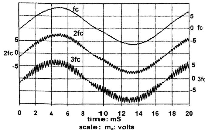
Fig. 6.3 Comparison between  $m_a$  signals:  $f_c = 2.5k Hz$ ,  $f_{20dB} = f_c, 2f_c, 3f_c$
