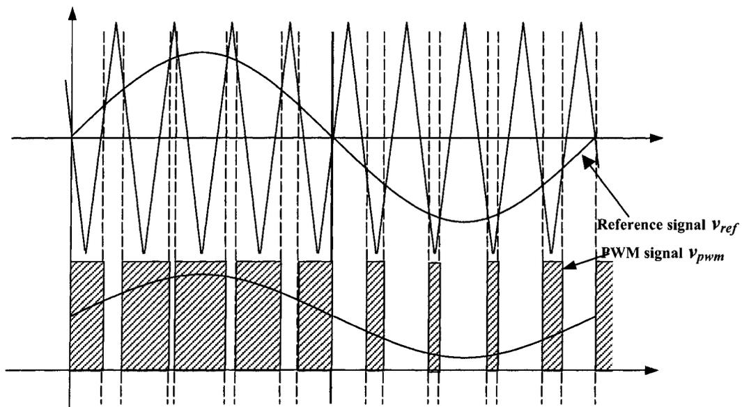
Fig. 1.3 Bipolar PWM switching waveforms
