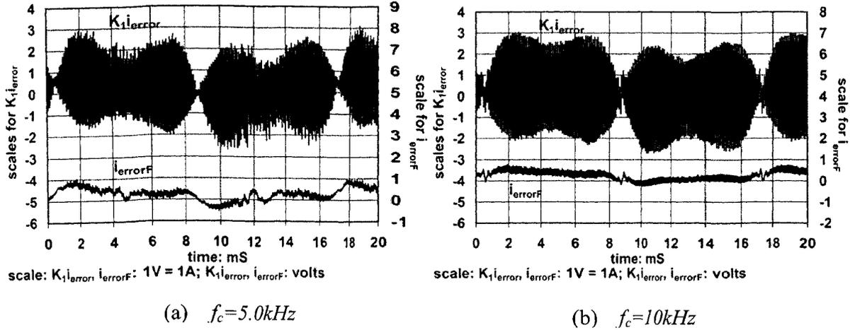
Fig. B.1 Experiment results of  $K_1 i_{error}$  and  $i_{errorF}$
