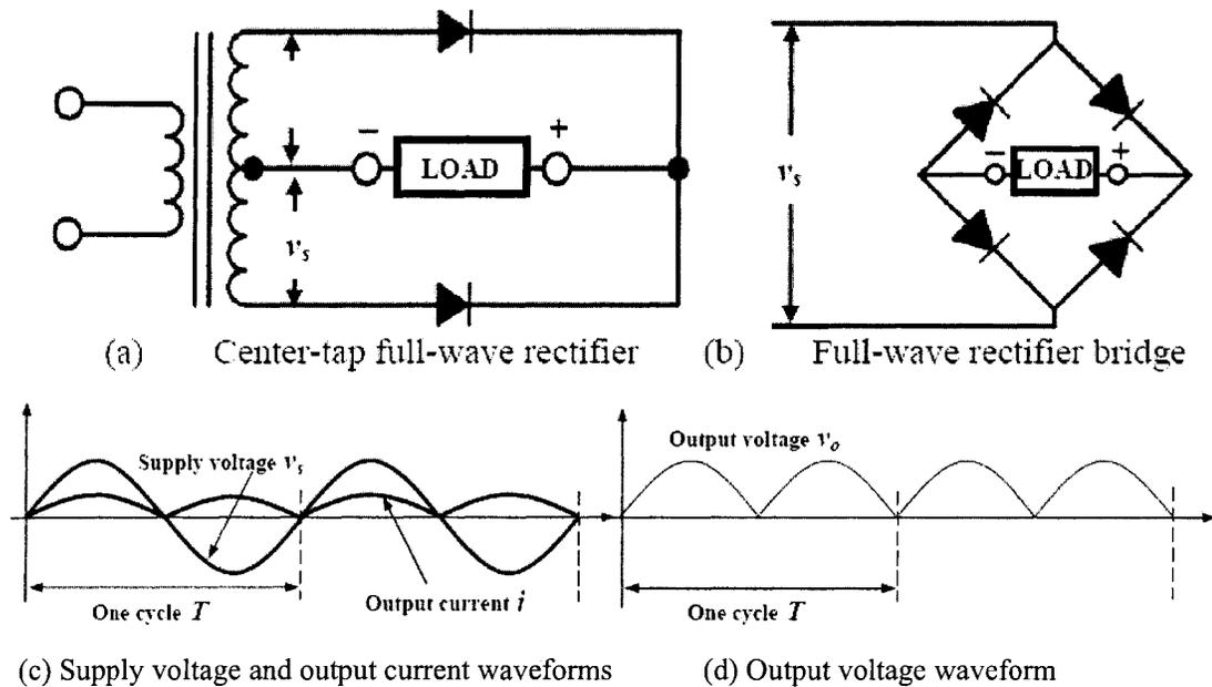
Fig. 1.8 Circuits and waveforms for full-wave rectifier
