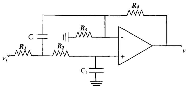
Fig. 5.11 A second-order VCVS low-pass filter
