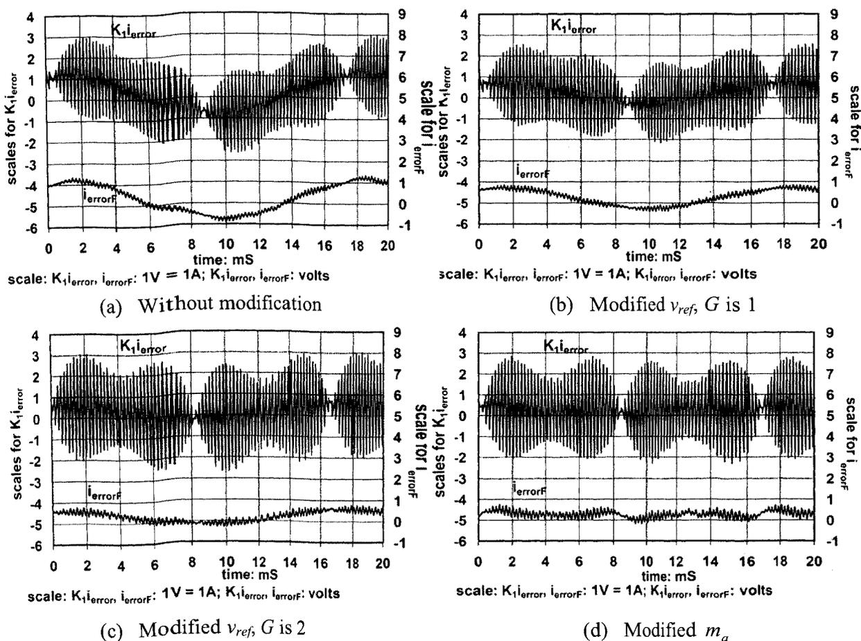
Fig. 6.12 Experimental waveforms of 2 techniques for lowering the average current error signal
