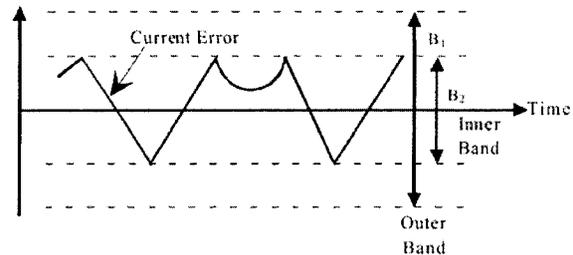
Fig. 2.5 Double hysteresis band current control
