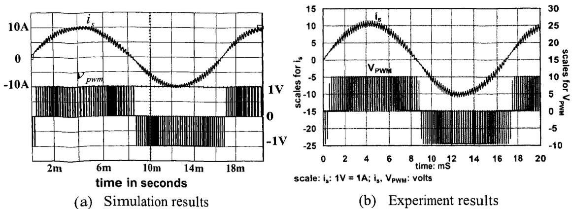
Fig. 6.2 Simulation and experiment results comparison between  $i_s$  and  $v_{pwm}$
