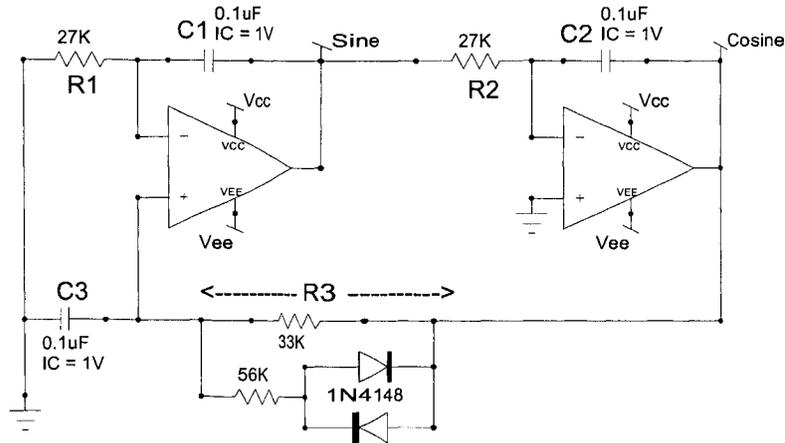
Fig. 5.15 The sinusoidal waveform oscillator
