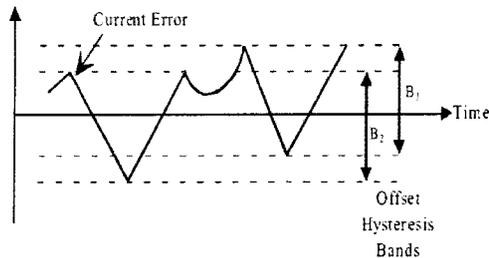
Fig. 2.4 Three level multi-band hysteresis current control
