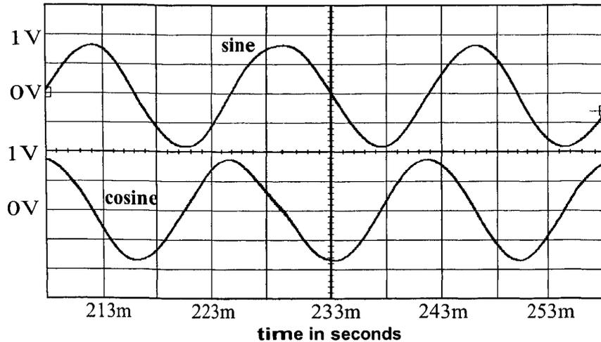
Fig. 5.16 The output wave forms of the oscillator: sine and cosine
