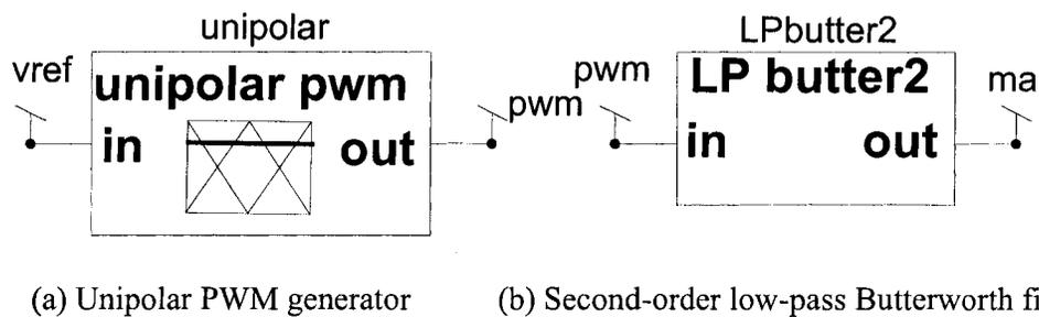
Fig. 4.2      Function block of PWM generator and filter
