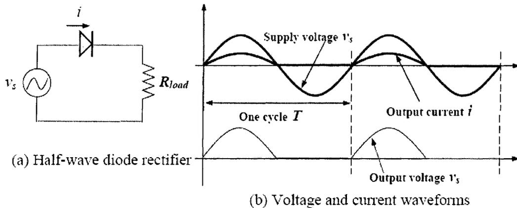
Fig. 1.7 Circuit and waveforms for single-phase half-wave diode rectifier
