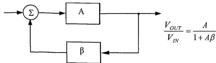
Fig. 5.14 Canonical form of a feedback circuit
