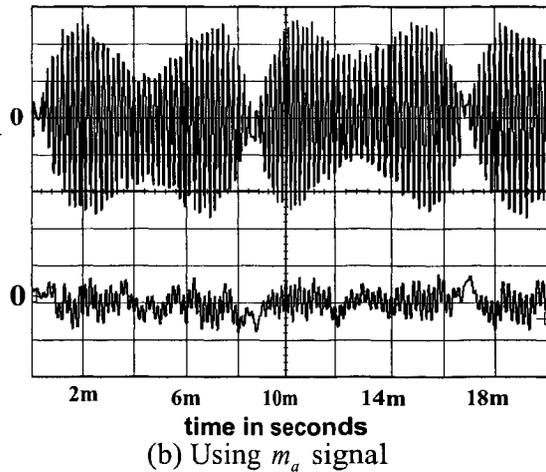
Fig. 4.15 Effect of using modified  $m_a$  to lower the pwm-cycle average current error: type-1 controller
