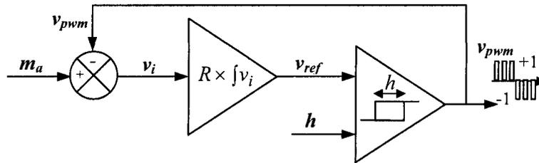
Fig. 3.1 Hysteresis PWM signal comparator
