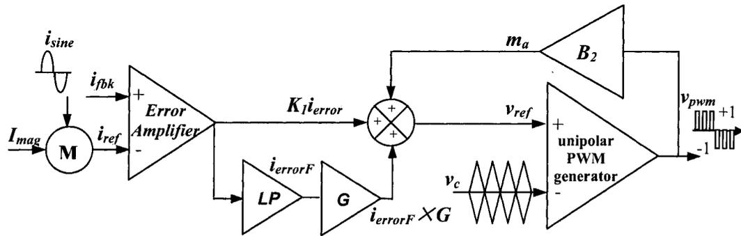
Fig. 3.11 Function block diagram for the type-1 current controller with the filtered current error signal
