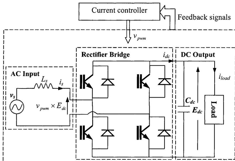
Fig. 1.9 Single-phase PWM current controlled rectifier
