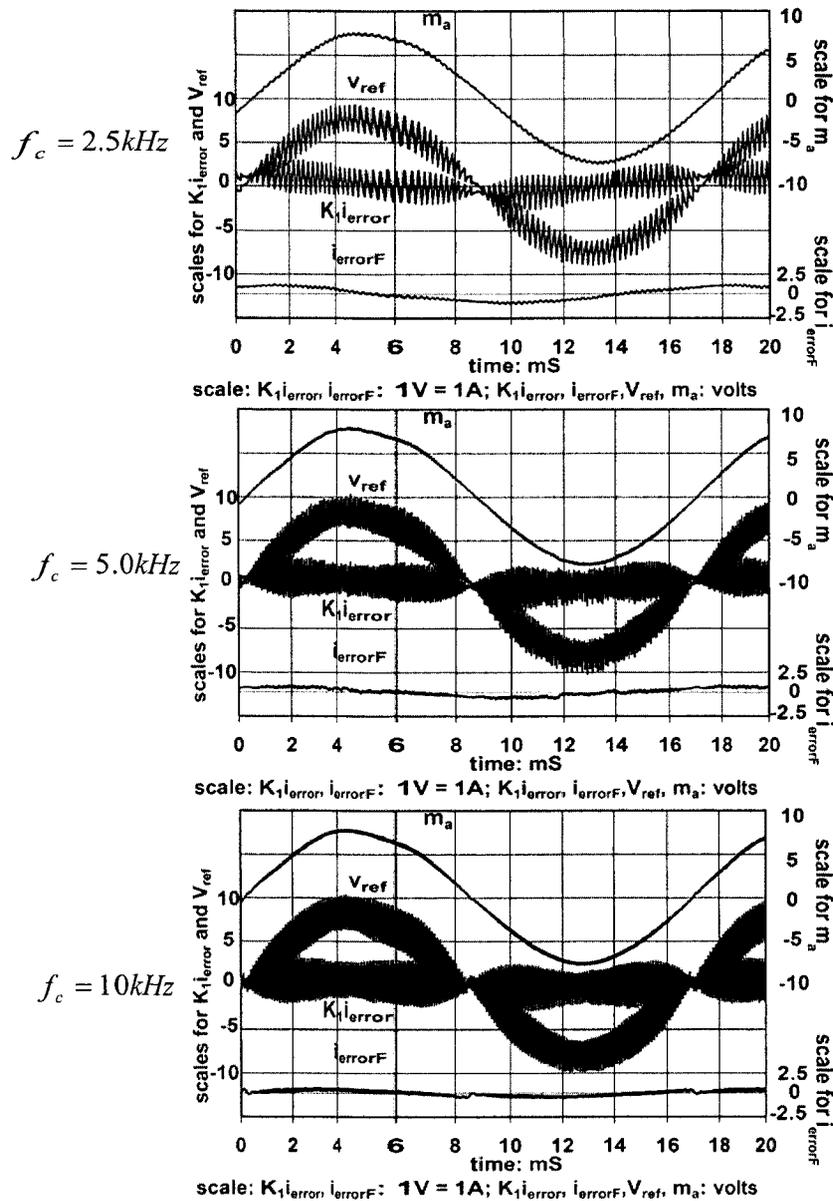
Fig. 6.5 Experiment results for type-1 current controller:  $f_{20dB} = f_c$ ,  $f_c = 2.5k, 5k, 10k$  Hz
