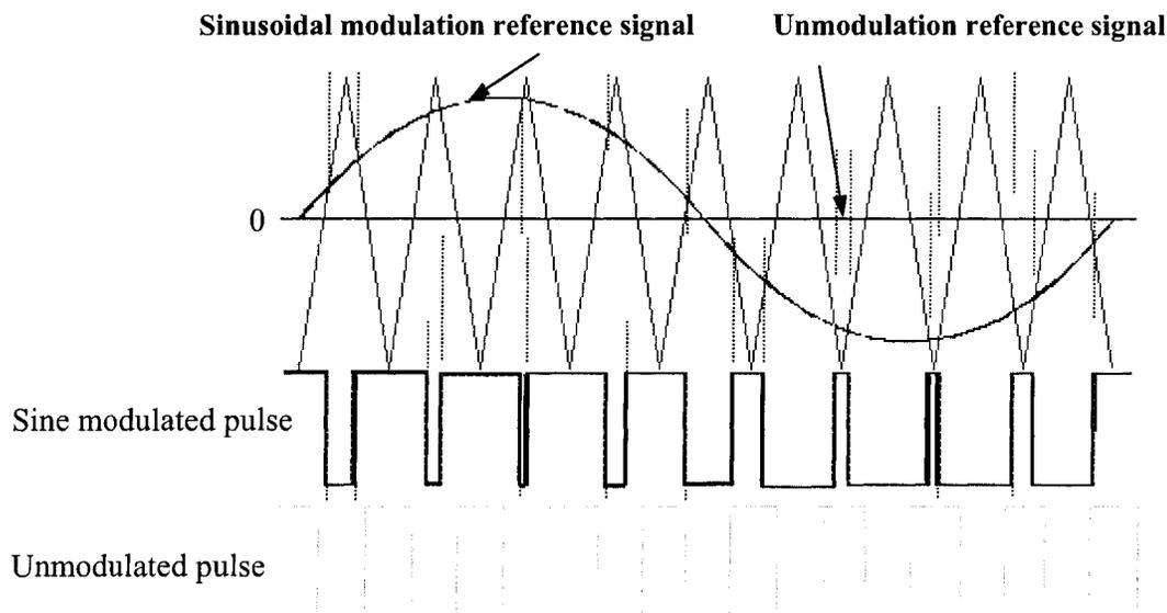
Fig. 1.2 Sinusoidal modulated and unmodulated pulse signals
