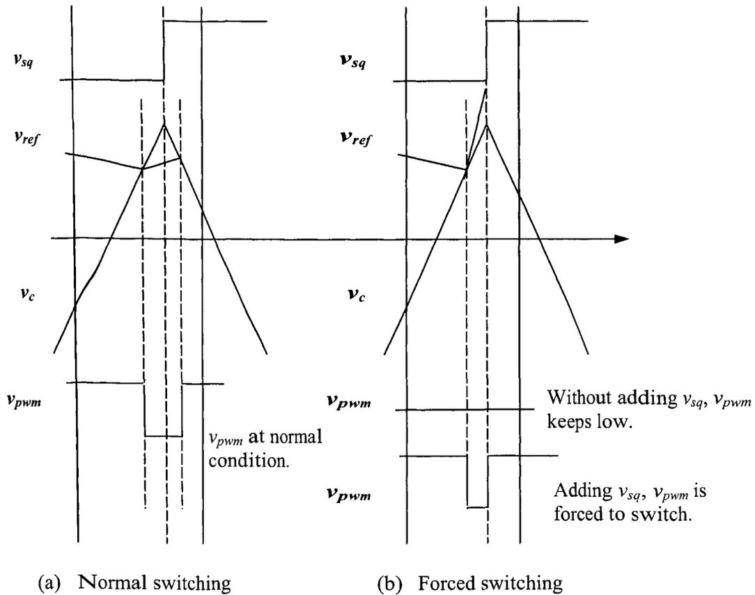
Fig. 5.8 Adding  $v_{sq}$  signal to avoid lost switching
