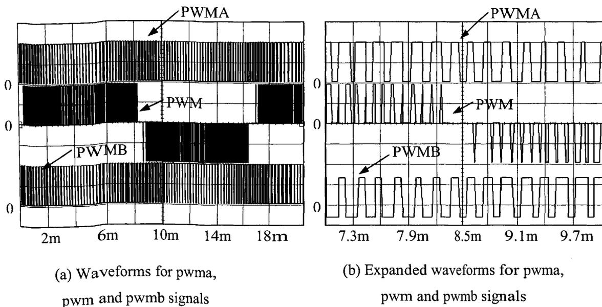
Fig. 5.9 Waveforms for pwma, pwm and pwmb signals
