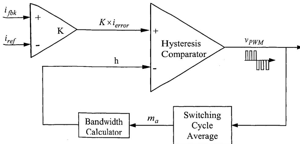
**Fig. C1 Block diagram for the digital controller**
