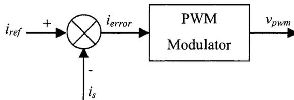
Fig. 1.10 PWM current controller
