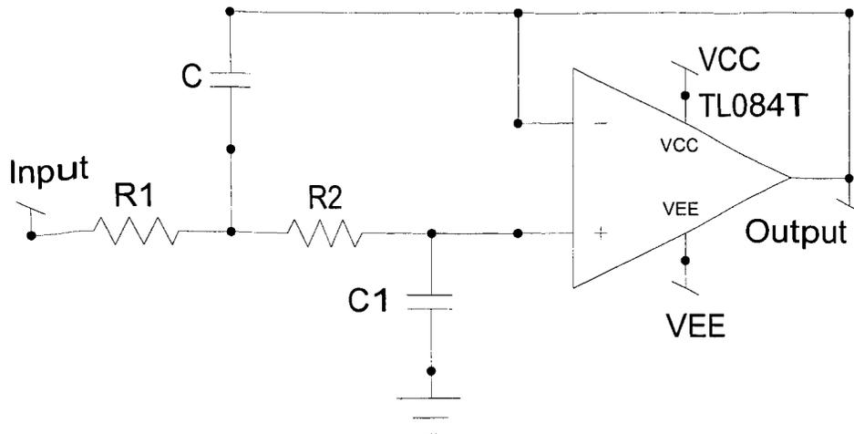
Fig. 5.12 A unit gain second-order low-pass Butterworth filter
