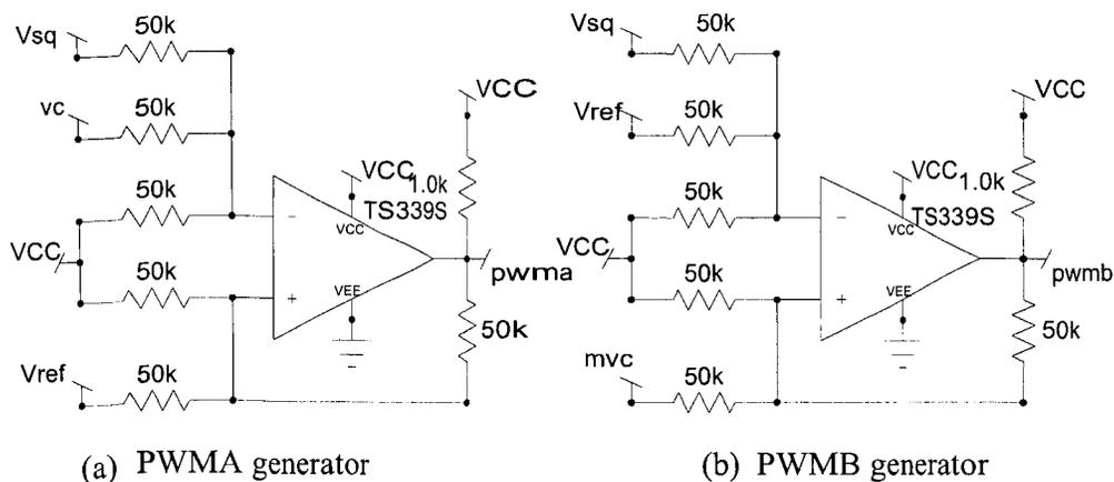
Fig. 5.7 PWMA and PWMB generator
