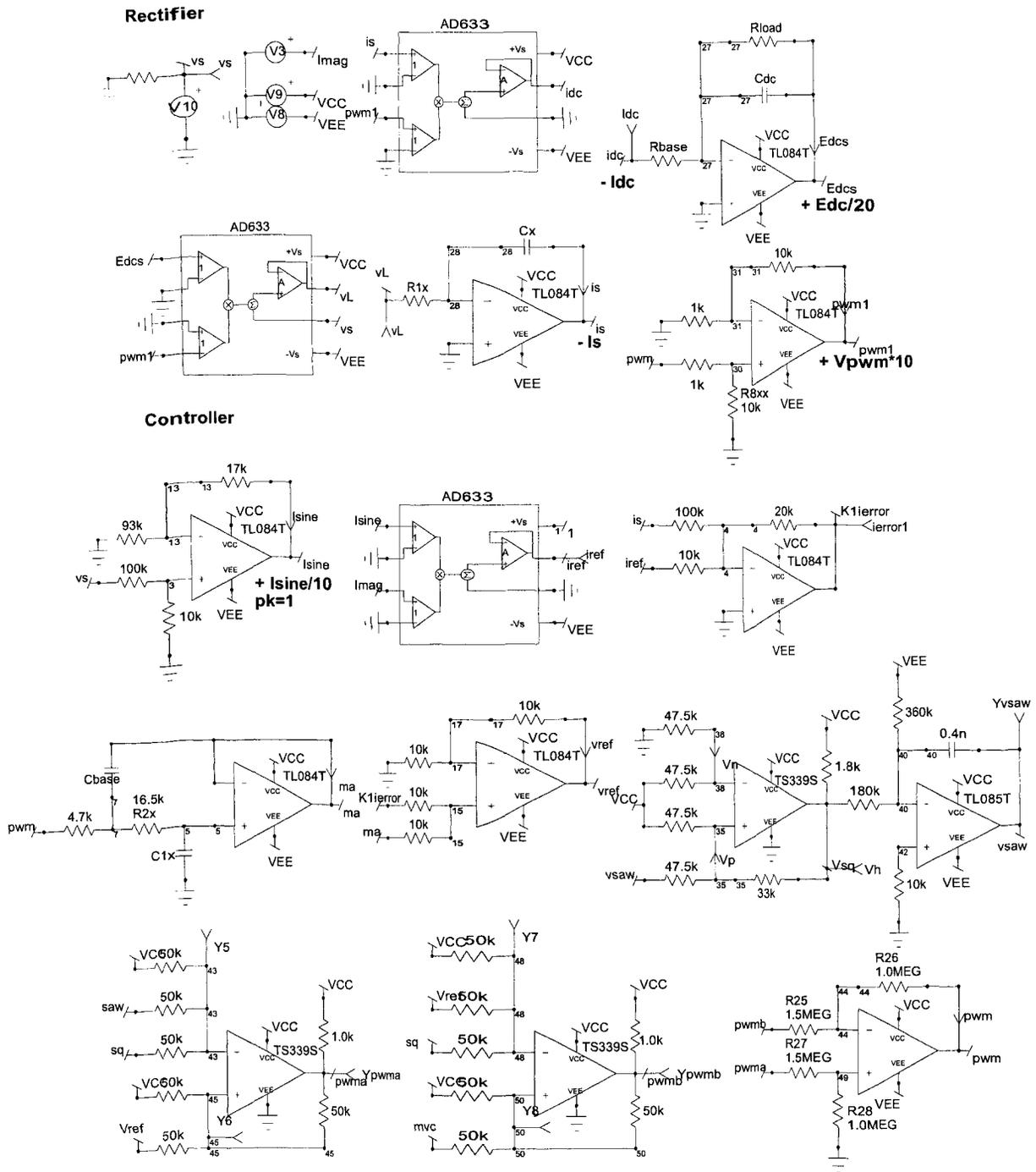
Fig. 5.3 Overall circuit for the type-1 current controller
