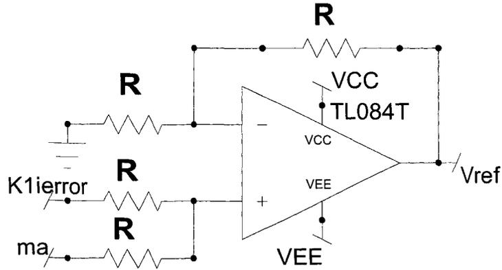
Fig. 5.10  $v_{ref}$  signal generator
