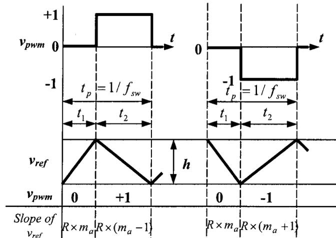
Fig. 3.2 Expanded waveforms of a delta-modulated hysteresis PWM controller
