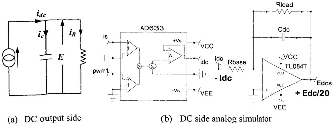
Fig. 5.2 DC side of the single-phase rectifier simulator
