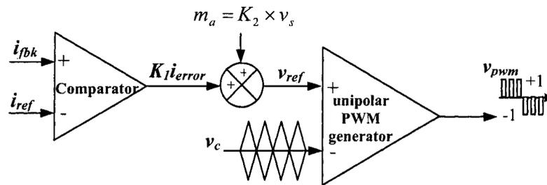
Fig. 3.6 Function Block Diagram for the carrier-based PWM current controller
