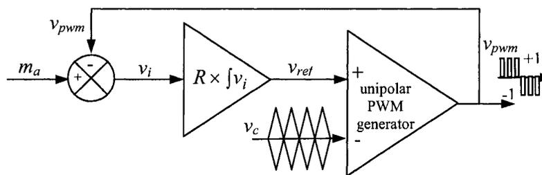
Fig. 3.3 Ramp comparing PWM signal comparator
