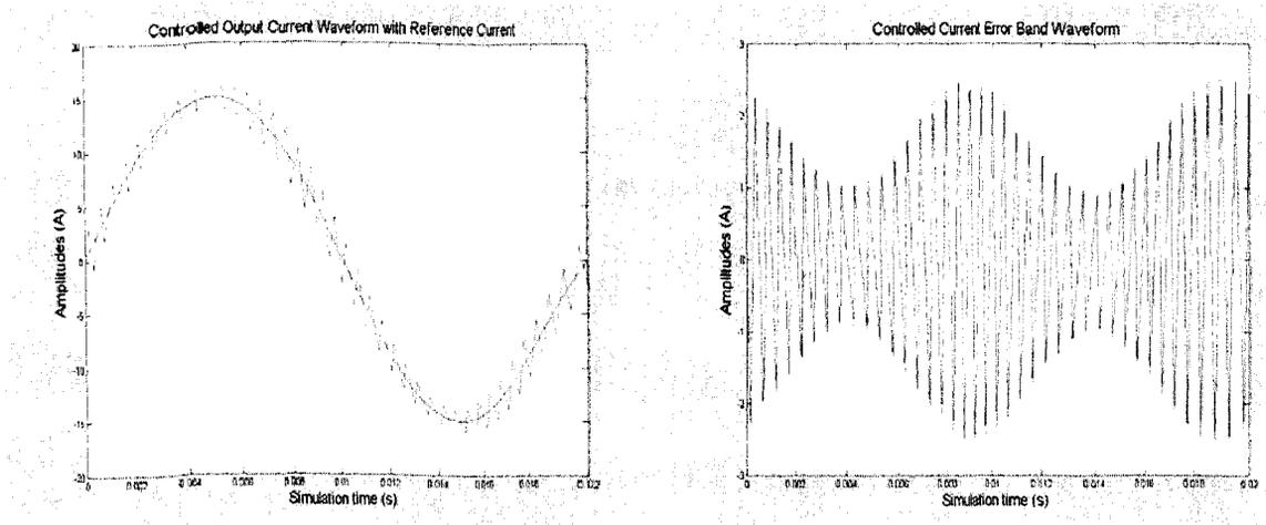
**Fig.C2 The output current and current-error**
