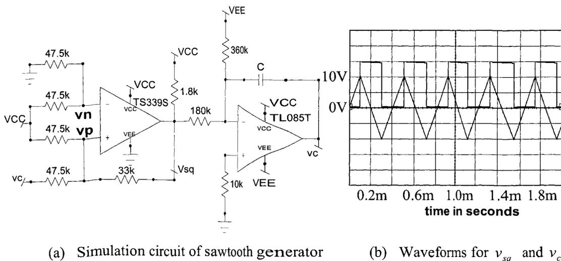
Fig. 5.4 The analog sawtooth generator:  $\pm 10\text{V}$  peak
