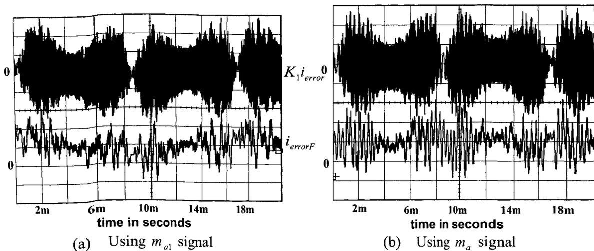
Fig. 4.17 Effect of using modified  $m_a$  to lower the pwm-cycle average current error:
