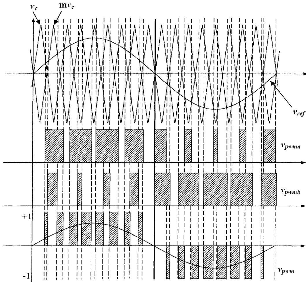
Fig. 1.4 Unipolar PWM switching waveforms
