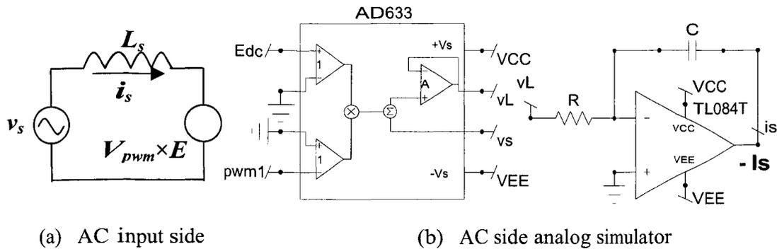
Fig. 5.1 AC side of the single-phase rectifier simulator
