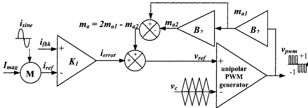
Fig. 3.12 Functional diagram for the type-1 current controller
