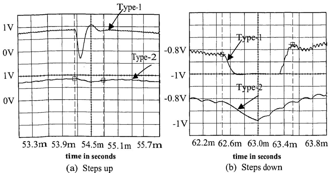
Fig. 4.20 Expanded waveforms for the transient response
