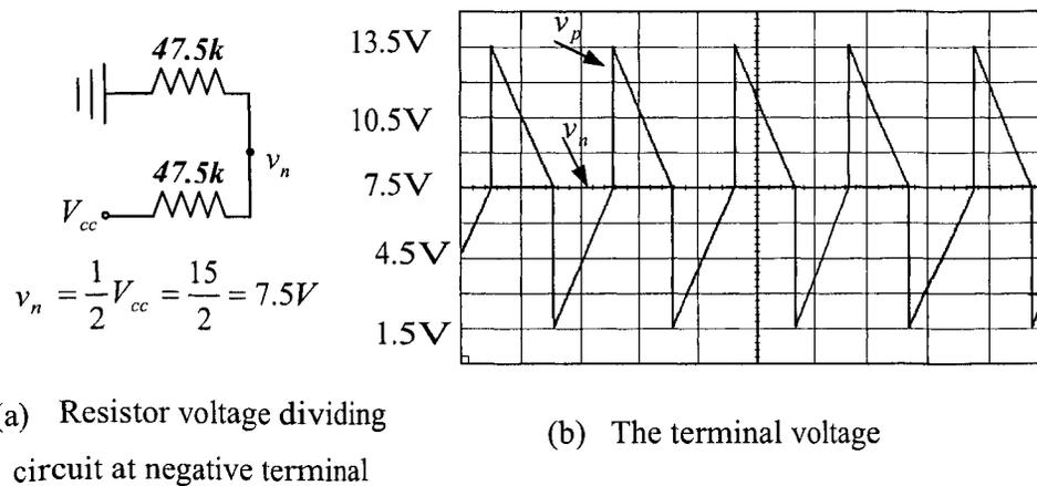
Fig. 5.5 Analysis of the comparator circuit and terminal voltage
