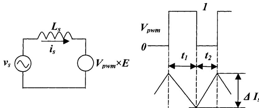
(a) The simplified AC input side (b) Waveforms of PWM signal and Current-error
