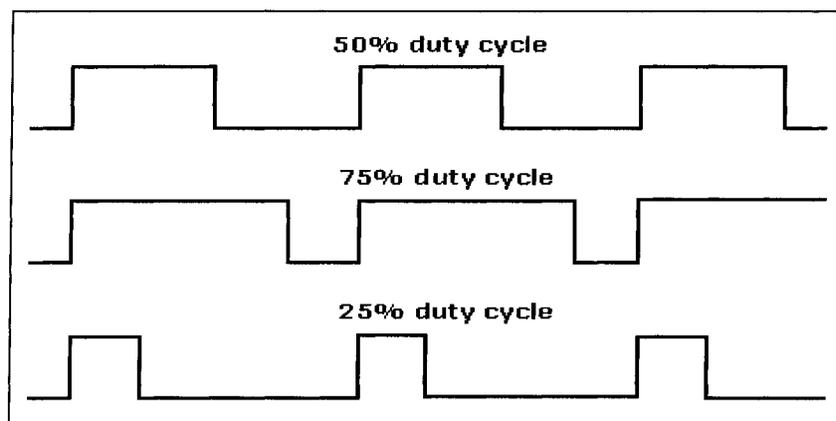
Fig. 1.1 Pulse width modulation waveforms
