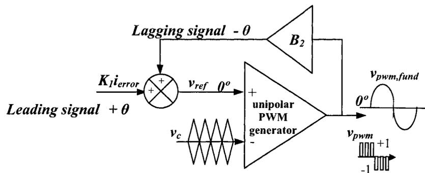
Fig. 3.10 Unipolar PWM comparator and signal phase angle analysis
