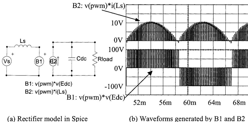
Fig. 4.1 Rectifier simulation model and waveforms
