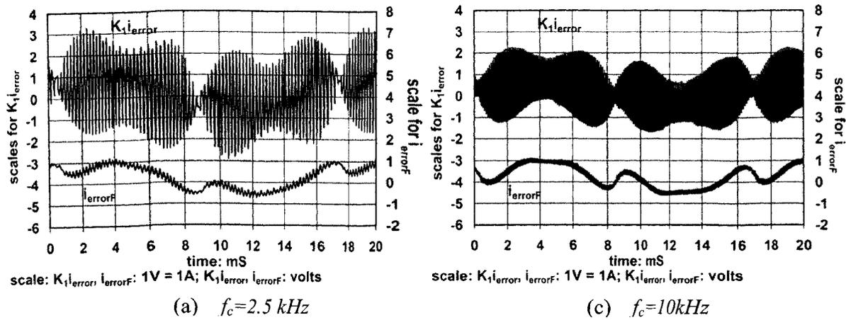
Fig. B.2 Experiment results of  $K_1 i_{error}$  and  $i_{errorF}$
