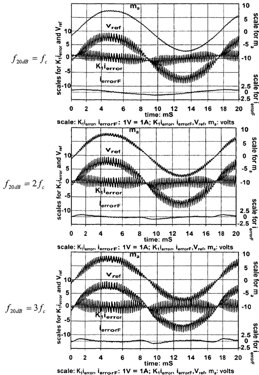
Fig. 6.4 Experiment results for type-1 current controller:  $f_c = 2.5k$  Hz,  $f_{20dB} = f_c, 2f_c, 3f_c$
