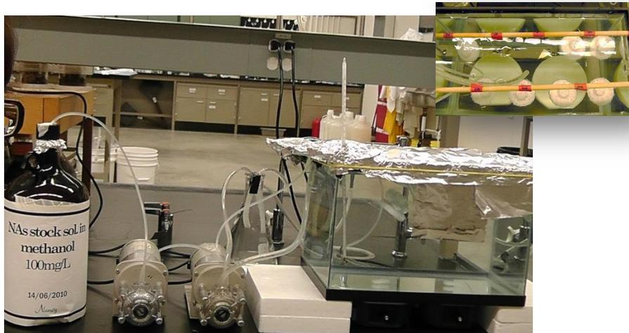
**Figure K- 6.** Flow-through system for integrative experiment
