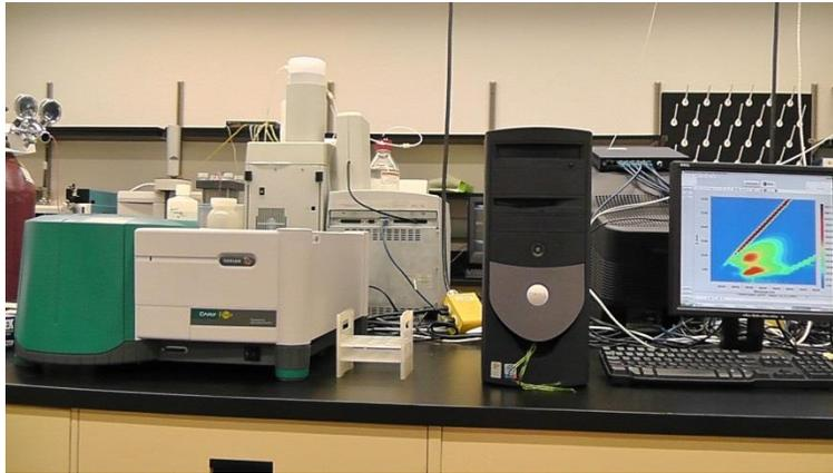
**Figure K- 1.** Varian fluorescence spectrophotometer
