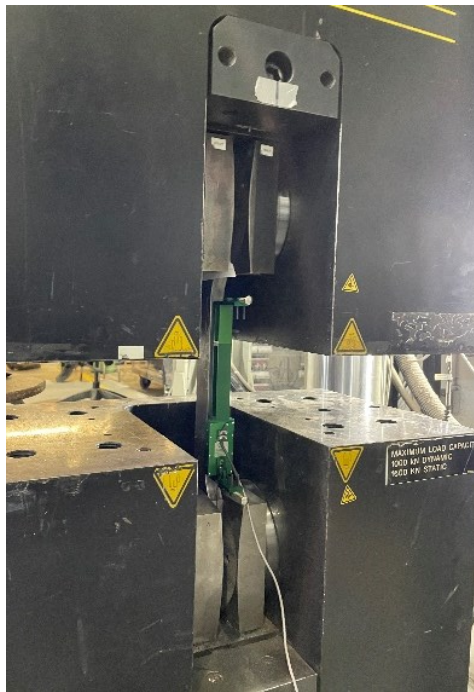
Figure C.3: Tension coupon in the test machine.
