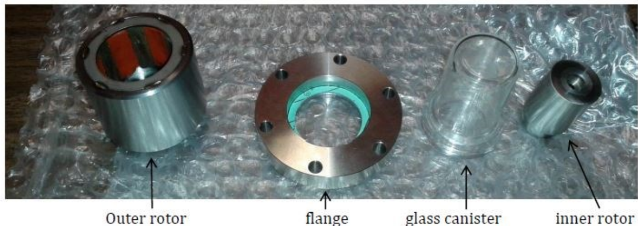
Figure 17: Magnetic coupling components. Outer rotor connects to the motor, inner rotor connects to the shaft. Flange and glass canister maintains the vacuum.
