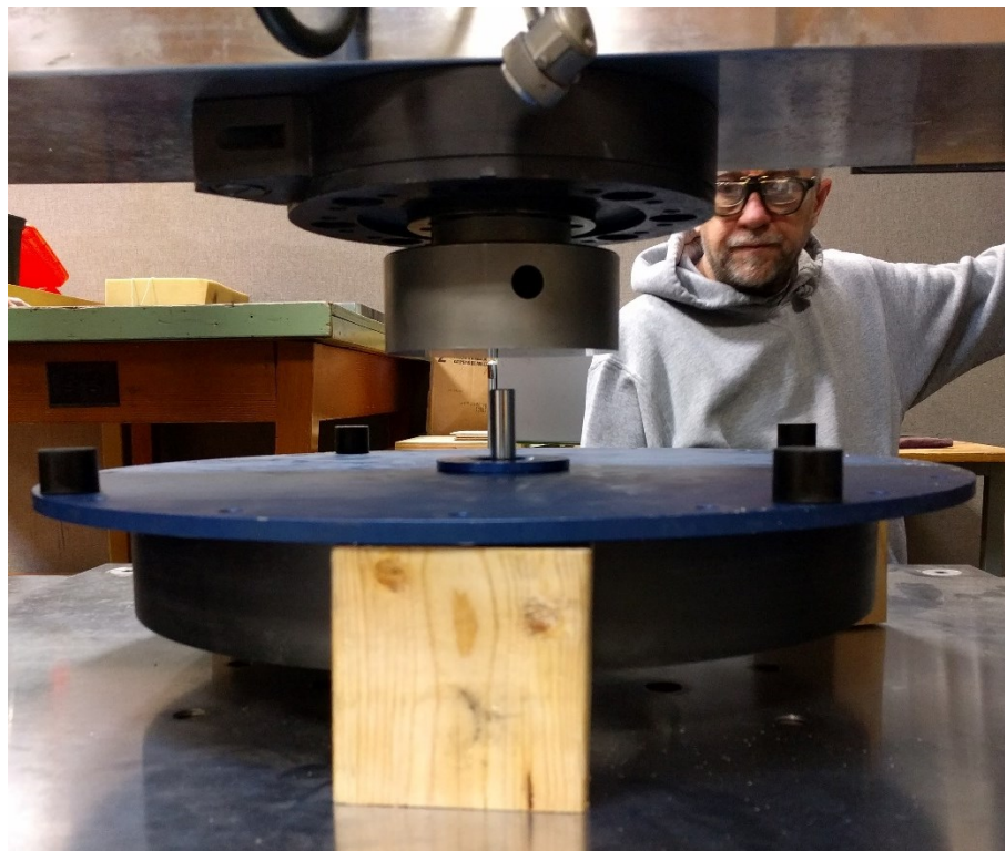
Figure 48: The rotor and bottom plate upside down in the press before the lower bearing is separated from the shaft.
