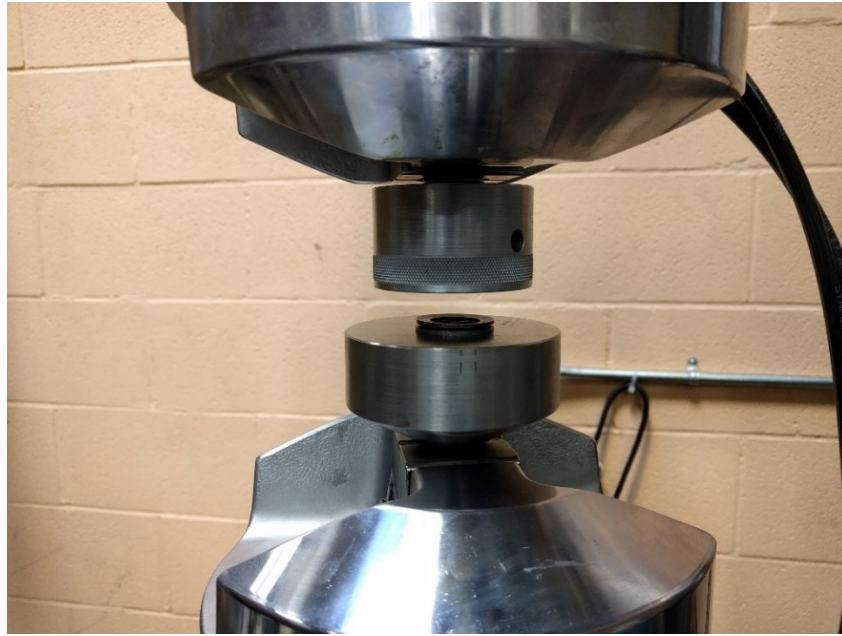
Figure 9: Test setup for compressive force of spring washers. The washers depicted here are in the second configuration, however the setup is the same for both tests. Same set up is used for magnets
